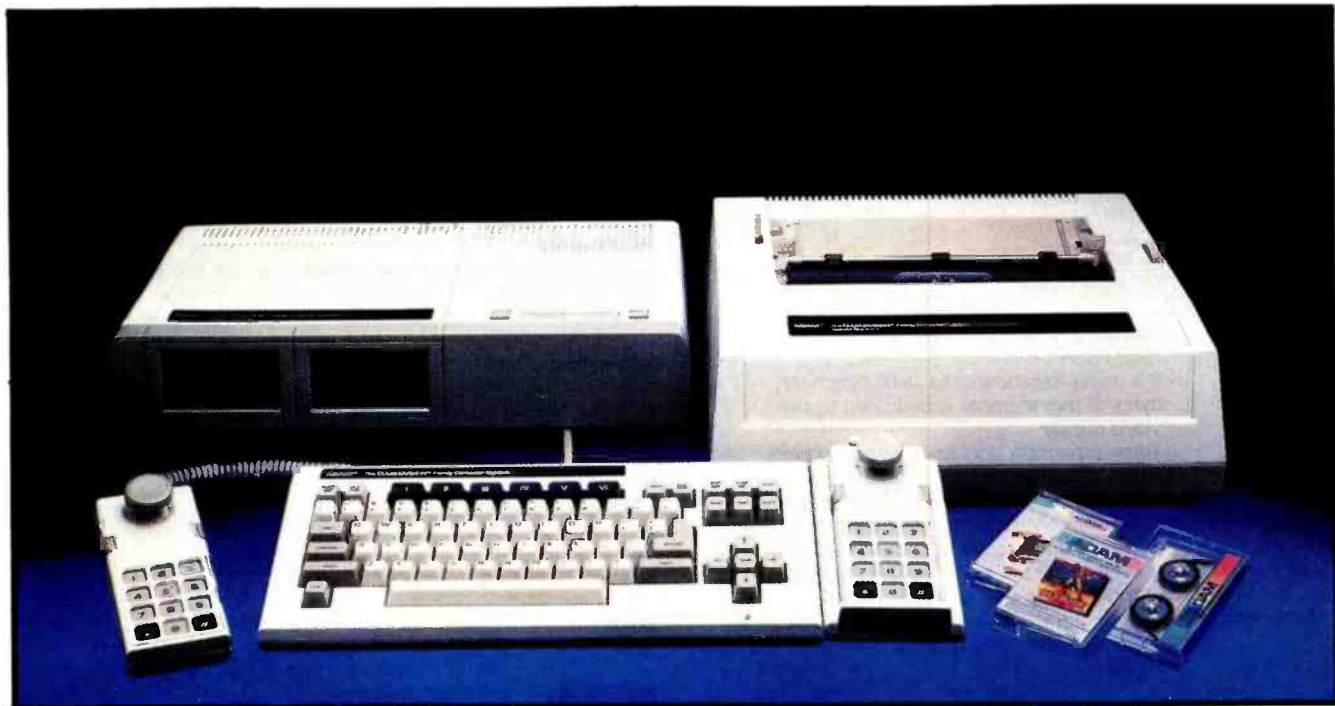
Photo 1: The Coleco Adam includes a tape drive, a printer, 64K bytes of RAM, a keyboard, a Colecovision game system, and two joysticks.
