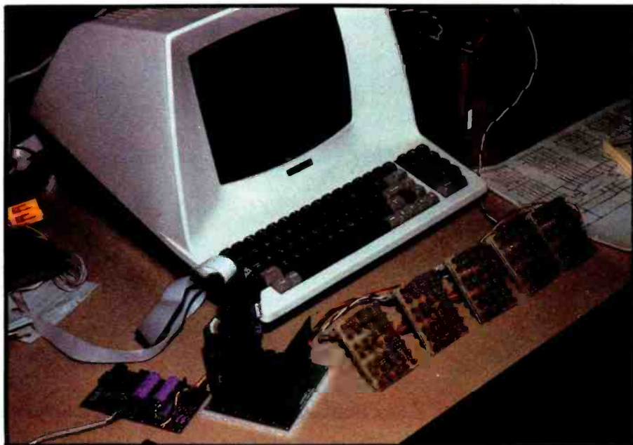
Photo 5: In my first attempt, several display segments were attached to the Z8 board; the message content of the display can be changed interactively from the video terminal.
