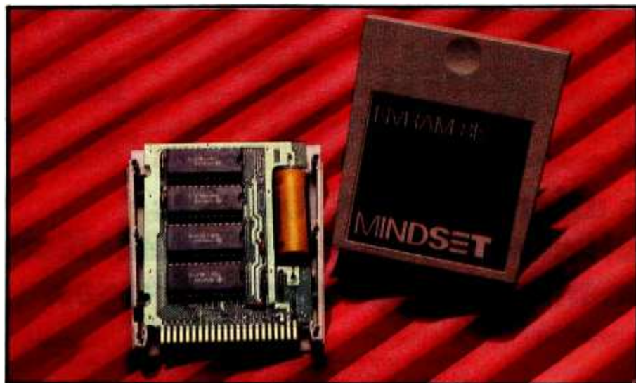
Photo 6: The Mindset RAM cartridge with battery backup. NVRAM stands for "nonvolatile RAM."
