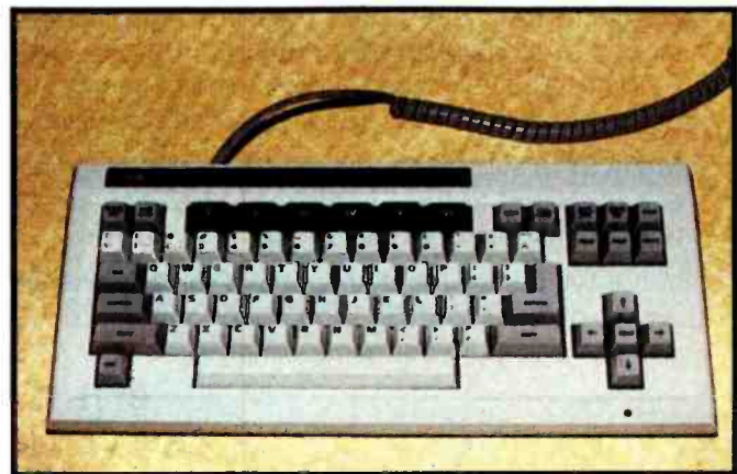
Photo 4: The Adam's detachable keyboard, perhaps the best-designed part of the system, has 75 full-travel keys.
