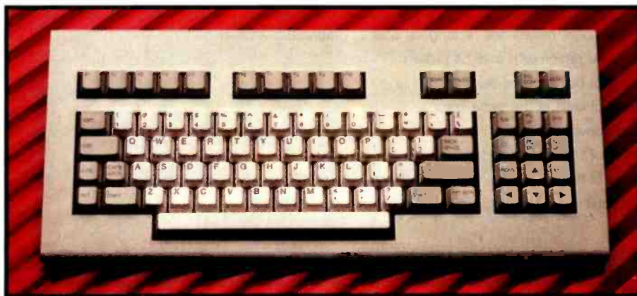
Photo 4: Although this Mindset keyboard is quite similar to the IBM PC keyboard, Mindset has made several improvements. Note, among other things, the more conventional layout of the function keys F1 through F10 and the improved position of the Shift keys.
