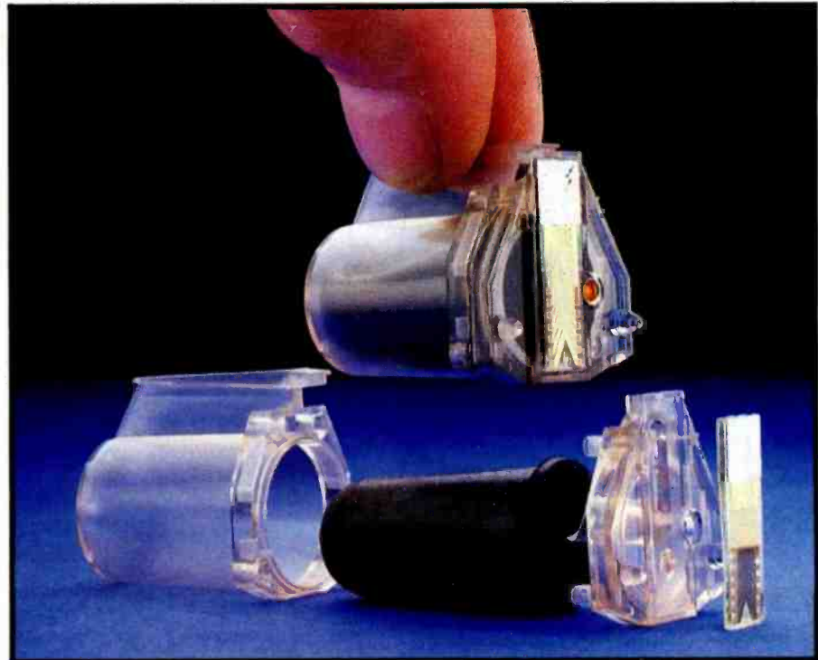
Photo 5: The simplicity of the HP 2225's print head is evident in this disassembled view. All the technology for printing is contained in the thin-film strip at the right.
