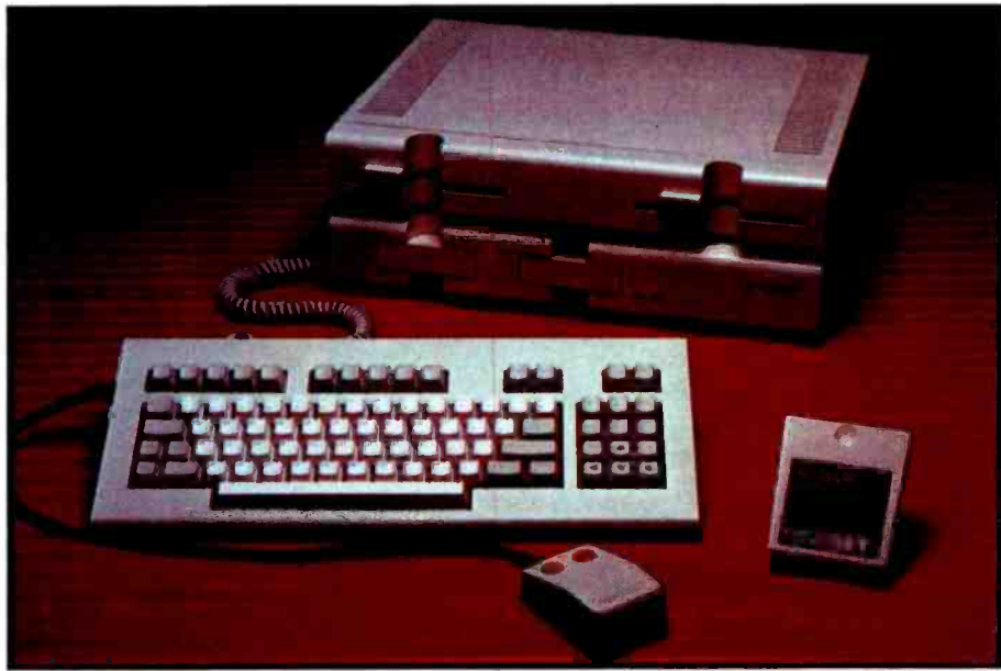
Photo 1: The Mindset Personal Computer. In the background are the System (bottom) and Expansion (top) units. In the foreground are the detachable keyboard, an optional two-button mouse, and the supplied GW BASIC programming language in cartridge form.
