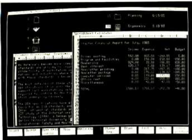
Photo 1: The workstation screen can be divided into several windows, each dedicated to a particular task. In the background window are the icons that represent various objects in the user's office. The two windows nearer the front are being used to work on a spreadsheet and a document. The labels on the softkeys at the bottom of the screen allow the user to select functions to be performed.
