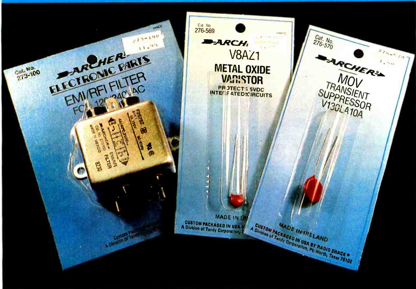
Photo 1: Your computers and other electronic equipment are vulnerable to disturbances transmitted through the power line. Most of the components necessary for transient and noise suppression can be purchased from Radio Shack. Shown here are a commercial EMI/RFI line filter made by Corcom and two General Electric metal-oxide varistors.
