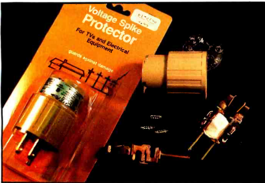
Photo 7: For quicker and easier, though incomplete, protection, you can plug your computer into a simple voltage-spike protector such as the Radio Shack 61-2790. As you can see from the disassembled unit, the metal-oxide varistor (wrapped in fiberglass tape) is connected between only the hot and neutral lines (black and white). It has no varistor connection to the ground lead and therefore does not protect against common-mode transients.
