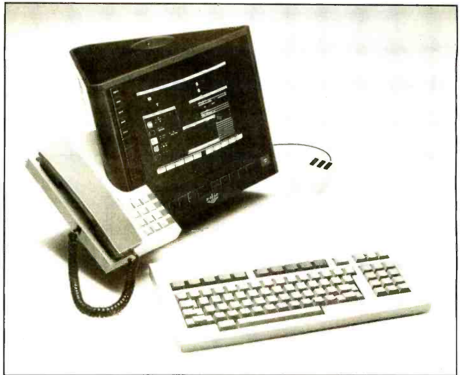
Photo 4: The Voicestation 1 provides the integration needed for office applications by combining a bit-mapped display and a telephone in a single compact unit. The workstation is connected to a central system over standard office telephone wiring.
