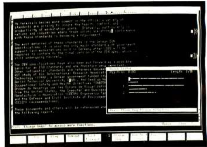
Photo 2: The small window in the foreground contains a visual representation of a recording made by the user. Solid lines show continuous speech, while breaks indicate pauses. The numbers mark reference points selected by the user. By moving the cursor around this display and using INSERT and DELETE keys on the keyboard, the user can edit the recording.
