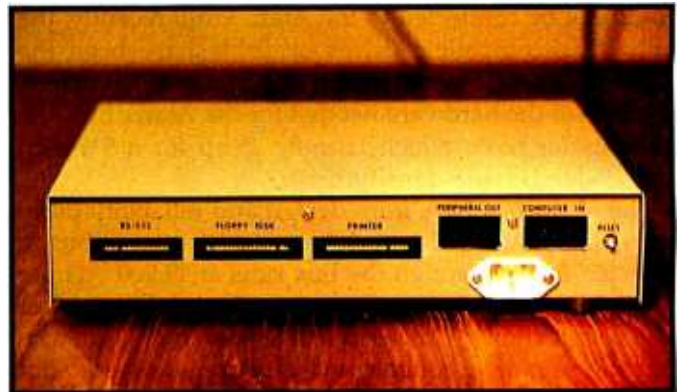
Photo 1: Front (a) and rear (b) views of the ATR8000. The rear connections shown in photo 1b are, from left to right, an RS-232C serial I/O port, a 34-pin floppy-disk connector, a 34-pin parallel printer port, and Atari serial I/O daisy-chain-out and -in connectors. A Reset button is located to the right of the daisy-chain connectors; the power connector is located directly below them.
