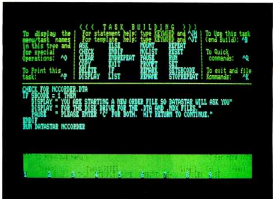
Photo 3: On this screen, the programmer specifies which actions will occur when an operator makes a menu selection. Although the final statement on the screen says to run Datastar, it could indicate any program.
