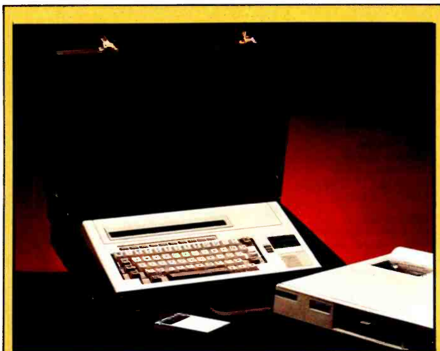
Photo 2: The Xerox 1800 portable computer is a custom version of the C8/16 computer system from Sunrise Systems. Note that the Xerox model uses the 80-character by 3-line LCD. The briefcase is optional.
