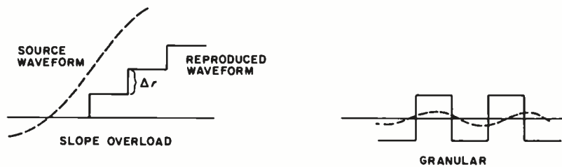
Figure 3b: Two potential problems occurring in delta modulation. When the source waveform changes too rapidly, the fixed quantization value may be too small to express the full change in the input; this slope overload causes a compliance error. Or when there is little change in the input waveform (at the extreme, a DC signal), vertical deflection in the quantization value results in granular noise in the output.
