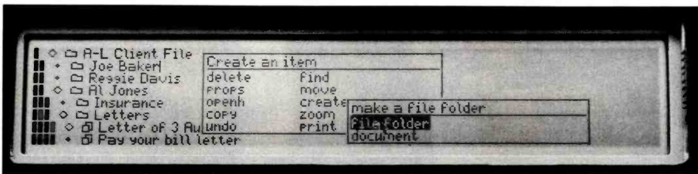
Photo 15: By pressing the Cancel area on the touch pad, you can return from the Help display to the desktop. The Create command is still active and you have a choice of creating a new file folder or document. The pointer is on file folder, and by tapping the touch pad, you can create a new folder.
