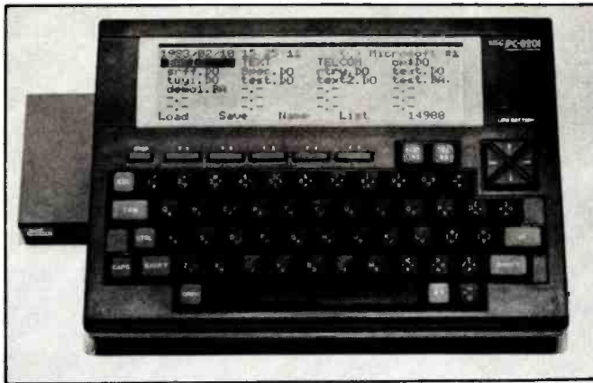
Photo 3: Screen display and keyboard layout of the PC-8201. Note that the keytop legends show both English characters and Japanese katakana characters. The special-function keys are labeled by the last line of the display.
