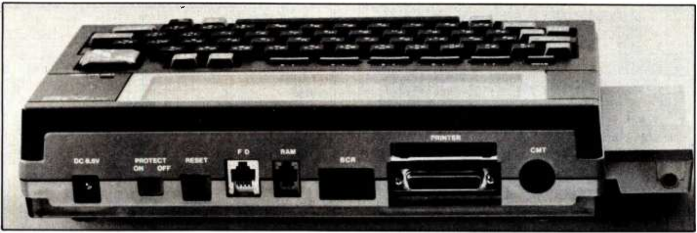
Photo 2: Rear view of the NEC PC-8201. From left to right are the AC power input jack, memory-protection switch, reset switch, and connectors for the floppy-disk controller (not yet released), memory-expansion modules, and bar-code reader. The Centronics-type parallel printer port is located above the RS-232C serial port, which is next to the cassette tape input/output port. An optional RAM cartridge is shown plugged into the side of the computer.
