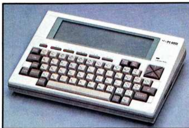
Photo 1: The NEC PC-8201 Portable Computer features a 40-character by 8-line LCD, software in ROM, and your choice of a red, white, or silver case.
