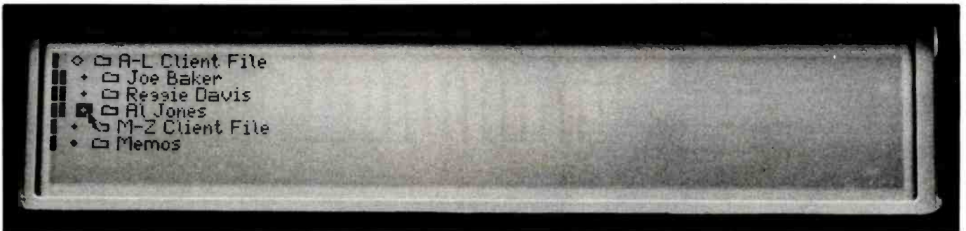
Photo 4: The A-L Client File is now open, and three files are shown inside it. Each of these three files is preceded by two bars, which indicate the level of nesting with the file drawer, and by the + sign that indicates a closed file. The operating system will open the Al Jones file, now highlighted, if you tap the touch pad.
