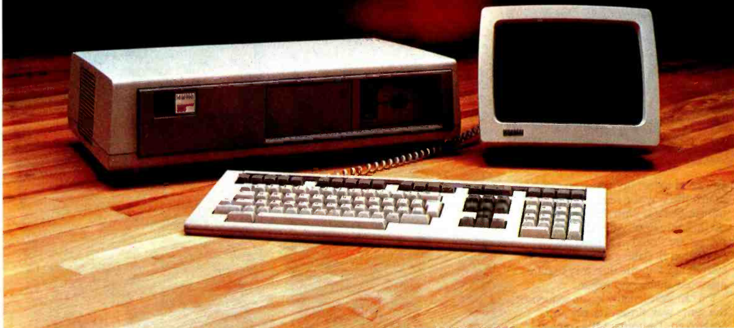
Photo 1: The Professional 300 Series includes both the Model 325 and the Model 350, the only differences being the number of available slots and the option of a Winchester hard disk.
