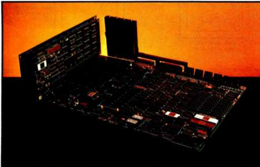
Photo 2: The main circuit board of the Fujitsu Micro 16s. Two processor boards are plugged into the expansion slots.
