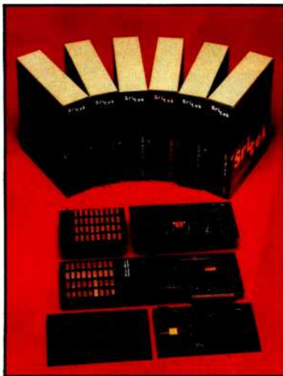
Photo 1: The Sritek modular expansion system for the IBM Personal Computer. The center circuit card is the Versacard, a 256K-byte dual-ported memory card that fits in a single slot of the IBM's expansion bus. Above it are a RAM Module (left), with an additional 256K bytes of memory, and a 68000 Microcard. Below the Versacard is a Z80 Microcard and an 8086 Microcard.
