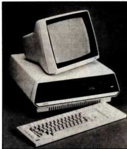
Photo 1: The new Altos 586 microcomputer offers affordable, fast 16-bit processing to accommodate five users, expandable to eight. The 586 uses the Xenix operating system and provides integral networking capability.
