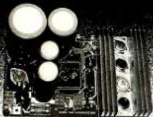
PS-101 Power Supply This solid supply gives you the capability of running any variety of 8" floppy or 5 1/4" floppy or hard disk drives as well as power a full S100-Buss
