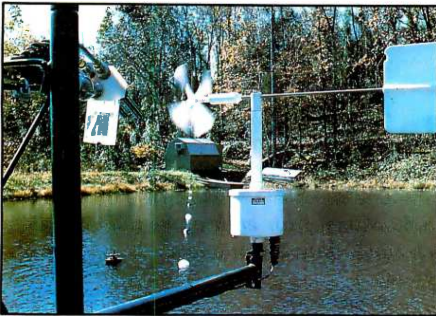
Photo 2: The buoys leading to shore support the wires that send analog signals to the cabin. The wire for transmitting the signals would have been the most expensive item of the whole installation if we had not bought it as military surplus.
