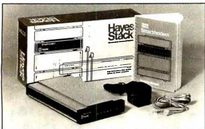
Photo 1: The Smartmodem package includes the modem, a modular telephone cable, an AC line adapter, and an excellent manual. (Photo by Ed Crabtree.)
