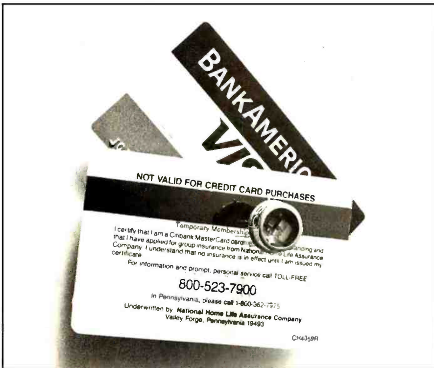
Photo 3: A common credit card could use the Drexon laser-recorded stripe. The stripe on the back of this card has a capacity of 1.6 million bits and is not susceptible to erasure by stray magnetic fields. A card this size completely covered on both sides could store 40 million bits. (Photo by Victor Budnik.)
