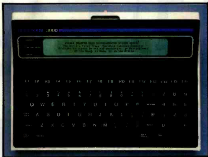
Photo 3: The T-3000's liquid-crystal display is the best around. The characters stand out clearly against a light, nonglare background.
