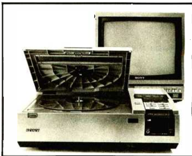
Photo 8: The Sony LDP-1000 (level-two) optical reflective videodisc player, which has a built-in RS-232C interface.
