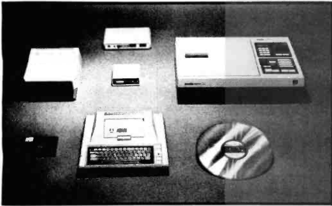
Photo 9: The Discmaster 5000 by New Media Graphics, a complete level-three system using the Pioneer VP-1000 and an Atari 400 computer.
