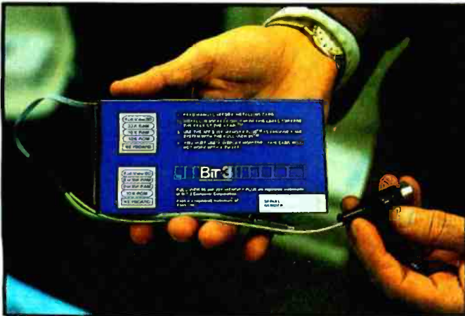
Photo 3: Full-View 80, an 80-column conversion board for the Atari 800, from Bit 3 Computer Corporation.
