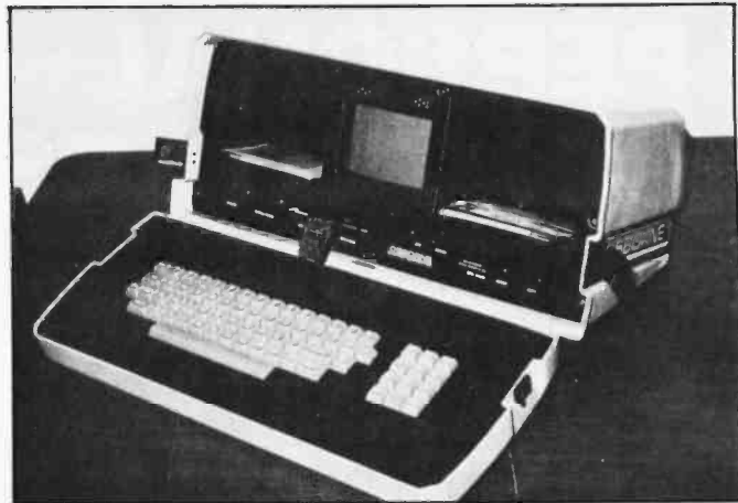
Photo 3: Front view of the Osborne 1. The 5-inch diagonal video display is seen at center, and the 5¼-inch disk drives are on either side of the display. Storage space for disks is provided below the two disk drives. RS-232C, IEEE-488, and modem cable connectors are in the lower left. An insulated ribbon cable connects the keyboard to the rest of the computer just below the video display. Brightness and contrast controls and external video connectors are found up front. The reset switch is also up front but is not likely to be pressed accidentally because of its location. The last connector is for the external battery pack.
