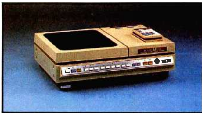
Photo 7: The Discovision Associates (DVA) PR-7820 "industrial" (level-two) optical reflective videodisc player. The DVA PR-7820's EPROMs have been updated twice (Models 2 and 3), resulting in faster search times and increased user-definable functions. Two-way communication between computer and disc is possible.
