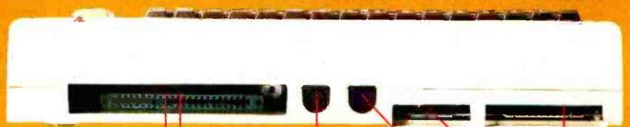
PLUG-IN PROGRAMS 3K/8K/16K MEMORY EXPANSION EXPANSION MODULE RF MODULATOR TELEVISION OR MONITOR VIDEO CABLE SINGLE DISK DRIVE COMMODORE DATACASSETTE MODEM FOR TELEPHONE AND TELECOMPUTING PRINTER
