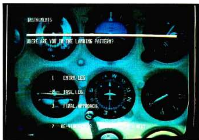
Photo 1: An "instrument tutorial" section of a low-cost flight-training system using the "overlay" interface, a TRS-80 Model III, and an optical videodisc player. The text, generated by the computer, is keyed directly over NTSC video (the flight instruments).
