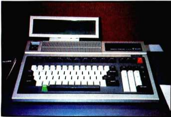
Photo 4: Toshiba surprised everyone when it previewed the T100 at the show. Shown here with the optional flat liquid-crystal display, the T100 is Z80-based and contains 64K bytes of user memory, 32K bytes of ROM, 16K bytes of video RAM, and provision for 32K-byte RAM and ROM packs. Toshiba will be offering Wordstar, dBase II, and all of the Structured Systems Group software, as well as CP/M, when the unit is officially introduced at next month's National Computer Conference in Houston.
