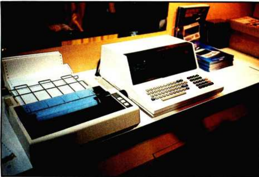
Photo 1: Casio's FX-9000P personal computer was finally introduced at the January Consumer Electronics Show. Using a Z80 look-alike, the basic unit comes with 12K bytes of ROM and one 4K-byte CMOS RAM pack with battery backup. RAM is expandable to 32K bytes, and a 16K-byte dynamic RAM pack is also available. The button-type keyboard contains only 67 keys but allows one-key access to many scientific and statistical functions. The printer is manufactured by Epson.
