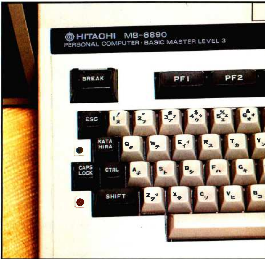
Photo 12: The Hitachi BREAK key is protected by a transparent plastic clamshell. The KATA/HIRA key can change the machine between any of three states—the color of the LED beside it indicates the state.
