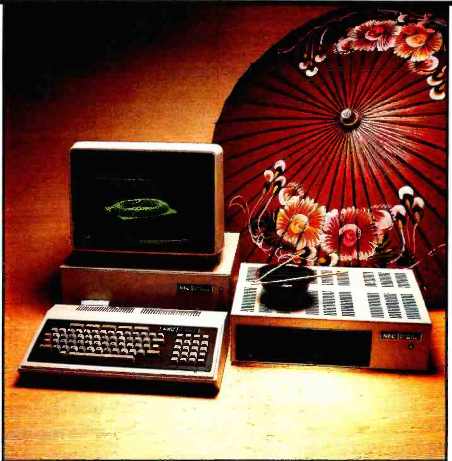
Photo 7: NEC's PC-8001A together with the color monitor, PC-8012 I/O unit, and PC-8032 dual floppy-disk drive.
