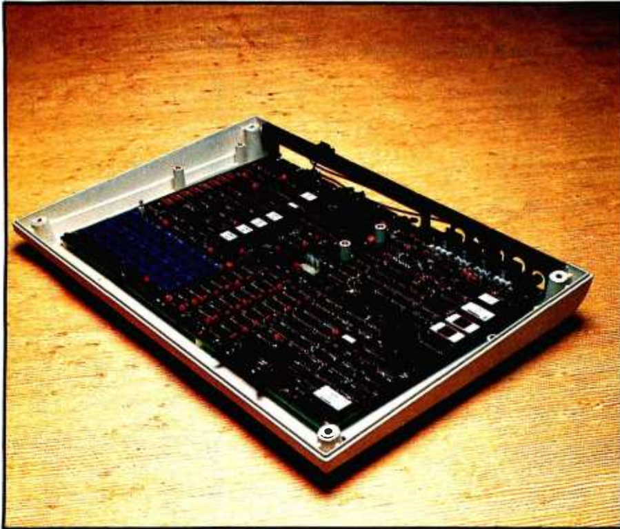
Photo 14: Inside the keyboard of the FM-8. Visible in the lower left are 16 ROM sockets for the alternate-character-set ROMS.
