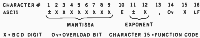
Figure 12: The BCD message format is a floating-point number in scientific notation followed by a comma, an overflow character, a function code, and a linefeed terminator. The floating-point number is represented by a sign, a mantissa, an "E" which indicates that an exponent follows, an exponent sign, and an exponent. Unused BCD digit inputs may be grounded; they will then be transmitted to the computer as 0s.
