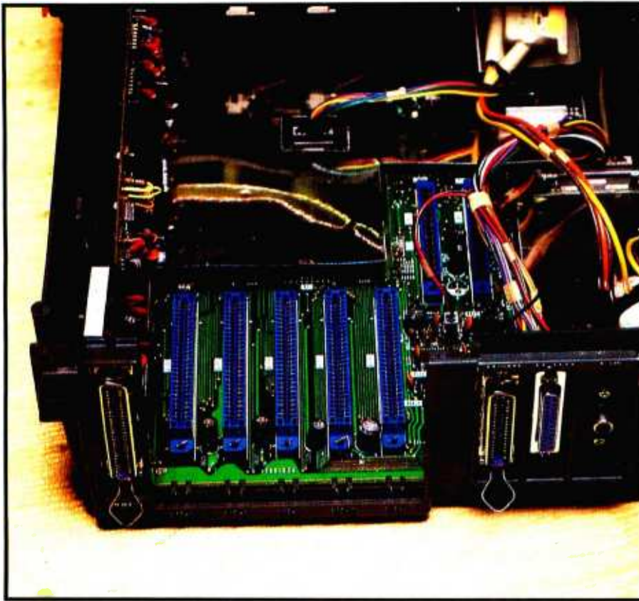
Photo 11: Hitachi provides a set of individually removable panels along the back of the processor enclosure to give access to individual expansion slots on the motherboard.
