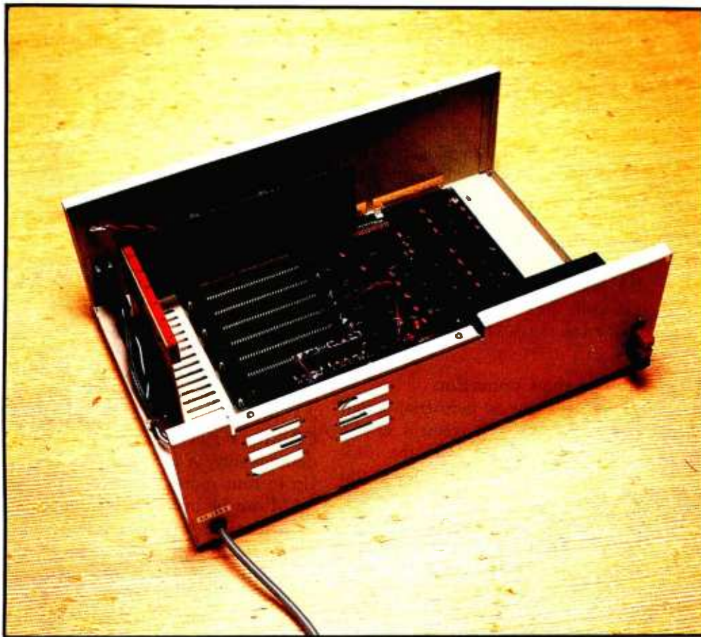
Photo 9: The NEC PC-8012A I/O unit has seven slots for expansion and connectors on the back that can carry nonstandard voltages to the bus.
