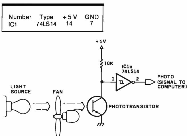
Figure 1: A sensing circuit for measuring rotational speed. The blades of the fan cast a shadow on the phototransistor as they pass between it and the light; the signal thus created is conditioned by a 74LS14 Schmitt trigger prior to being presented to the computer.
