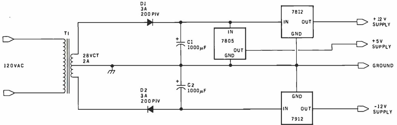
Figure 1: Simple and inexpensive power supply for the Z80 Starter Kit. It will provide +5 V at 1 A and  $\pm 12$  V at 200 to 300 mA for the Z80 Starter Kit and user circuitry. Parts used include: T1: 120 VAC primary, 28 VAC center-tapped secondary, 2 A; D1, D2: 3 A, 200 V PIV silicon diodes; C1, C2: 1000  $\mu$ F, 50 V electrolytic capacitors (note polarity carefully); 7805: +5 V, 1.5 A voltage regulator; 7812: +12 V, 1.0 A voltage regulator; 7912: -12 V, 1.0 A voltage regulator.
