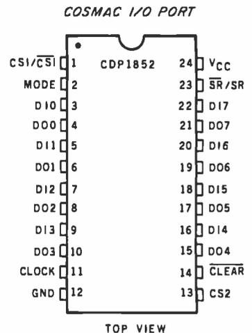
Figure 3: Pin assignments of the various integrated circuits used in the EPROM programmer.
