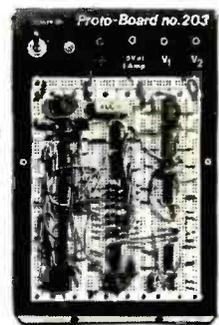
Fully assembled breadboard contains built-in, short-proof fused, 5VDC at 1 amp, regulated power supply. In addition to three QT-59S sockets, four QT-59B bus strips, one QT-47B bus strip and four binding posts. Capacity for most digital and many analog projects. **SIZE:** 9.75" Lg, 6.6" w, 3.25" h **WEIGHT:** 5 lbs.
