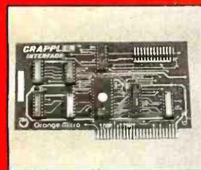
The Grappler™ interface card is the first to provide on-board firmware for Apple high resolution dot graphics. No longer does the user need to load clumsy software routines to dump screen graphics—it's all in a chip. Actually, it's our E-PROM, and it is replace-
