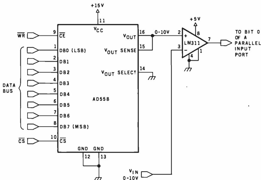
Figure 10: A software-driven 8-bit A/D converter.
