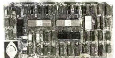
• Four buffered serial I/O ports • On-board Z-80A processor • Four CTC channels • Independently programmable baud rates • Vectored interrupt capability • Up to 4K of on-board PROM • Up to 2K of on-board RAM • On-board firmware
