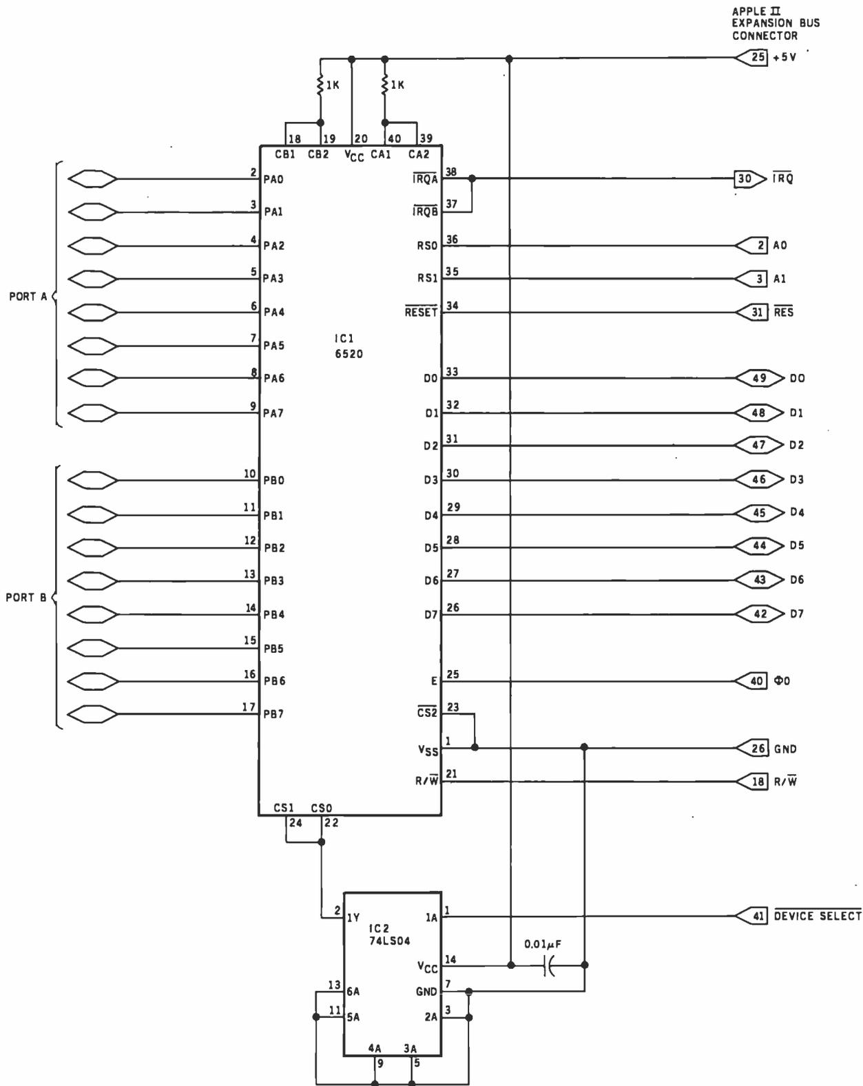
Figure 1: Interfacing an Apple II to a 6520 peripheral interface adapter. The active-low select line of the 6520 is tied to ground while both active-high select lines are connected via an inverter to Device Select (an active-low signal generated by the Apple II that enables one of its eight peripheral positions).
