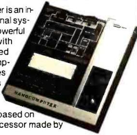
**POWERFUL** — based on the Z80 microprocessor made by SGS-ATES
