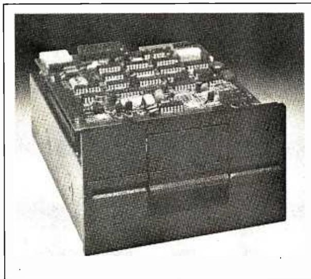
sity: 48 TPI • Cylinders: 35 or 40 • Tracks: 70 or 80 • Recording Method: FM or MFM • Rotational Speed: 300 RPM • Transfer Rate: 250K bits/second • Latency (avg.): 100 ms • Access Time: Track-to-track 12 ms; Settling 15 ms • Head Load Time: 50 ms
