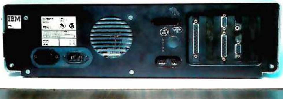
Photo 10: The back panel of the IBM Personal Computer. See the text for a description of the plugs and sockets.
