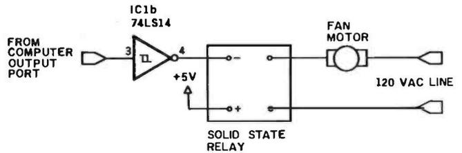
**Figure 2:** The interface used to turn the fan motor on and off. A solid-state relay is simply driven from the computer's output port via a 74LS14 Schmitt trigger. This circuit is used in conjunction with the one shown in figure 1 to form a closed-loop control system. If the fan speed is too fast, the motor is turned off; if it is too slow, it is turned on.
