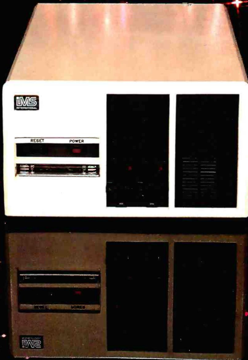
Configuration shown includes two slimline double sided, double density drives, 40 M byte Winchester subsystem with tape back-up.
