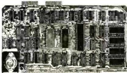
• S-100 bus compatible • Powerful 4MHz Z-80A CPU • Synchronous/asynchronous serial I/O port with RS-232 interface and software programmable baud rates up to 9600 baud • Parallel input and parallel output port • Four channel counter/timer • Four maskable, vectored interrupt inputs and a non-maskable interrupt • 1K of on-board RAM • Up to 32K of on-board ROM • System monitor PROM included
