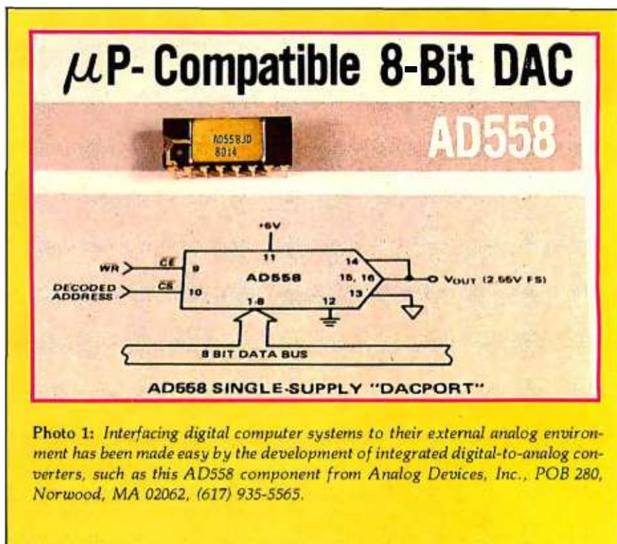
Photo 1: Interfacing digital computer systems to their external analog environment has been made easy by the development of integrated digital-to-analog converters, such as this AD558 component from Analog Devices, Inc., POB 280, Norwood, MA 02062, (617) 935-5565.
