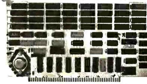
Enlarging the now "16K" ram chips, the Static 64 is the most current technology available in S-100 memory.
