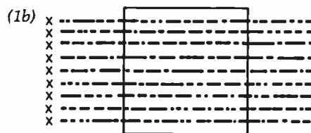
Figure 1: Figure 1a shows how screen data are normally organized. Horizontal scrolling can be accomplished by arranging the screen-data area as shown in figure 1b.
