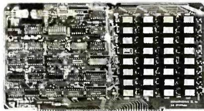
• S-100 bus compatible • Up to 4MHz operation • Expandable from 16K to 64K • Uses 16 x 1 4116 memory chips • Page mode operation allows up to 8 memory boards on the bus • Phantom output disable • Invisible on-board refresh
