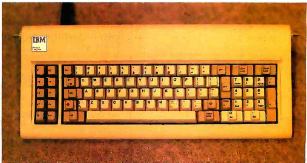
Photo 3: The IBM Personal Computer keyboard unit.
