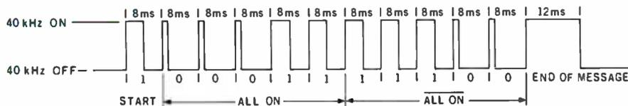
Figure 3: Data format for the ALL ON command. Note that the 5 command bits are complemented and repeated before the end-of-message pulse. Once a command or unit number has been sent, allow a 24-ms interval before the next transmission.
