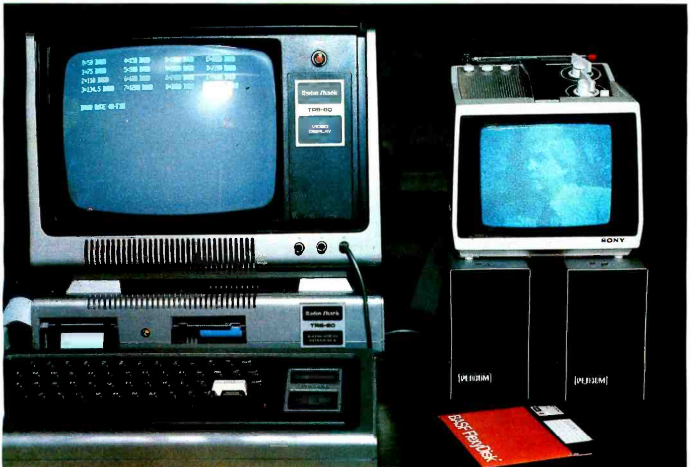
Photo 1a: To illustrate the effects of radiated and coupled interference, a portable TV set is placed next to an operating TRS-80 Model I computer. The result is a very snowy picture, primarily the result of radiated noise. Also note a slight blurring of the characters on the TRS-80 display screen. A beat frequency caused by magnetic coupling between the two video displays causes the TRS-80 screen image to shake. In a longer exposure, the characters would be illegible.
