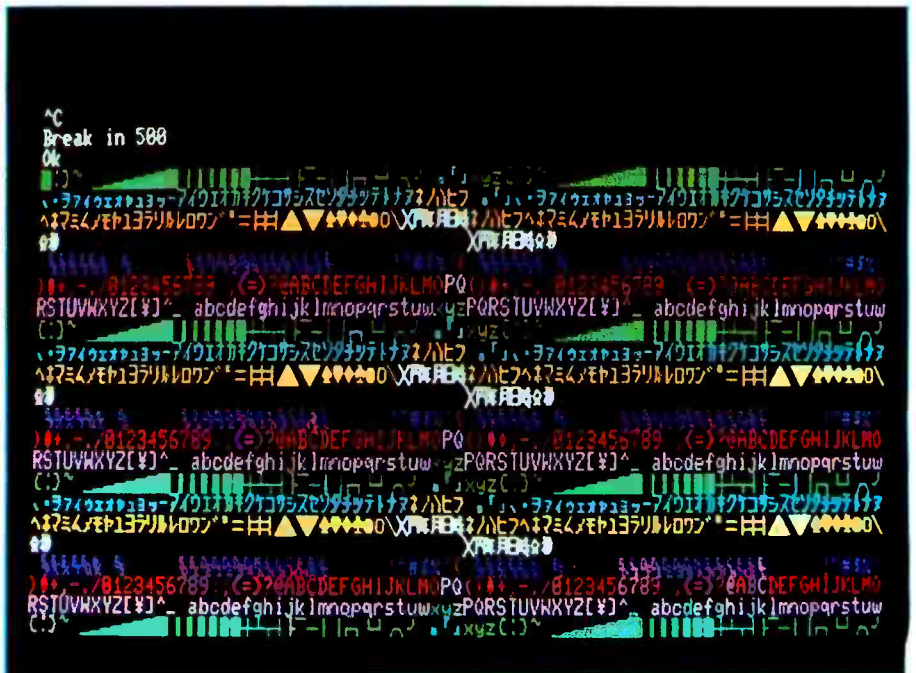
Photo 2: A display illustrating the colors and the character set on the PC-8001. In addition to complete ASCII, there are various graphics characters, control characters, and katakana characters.
