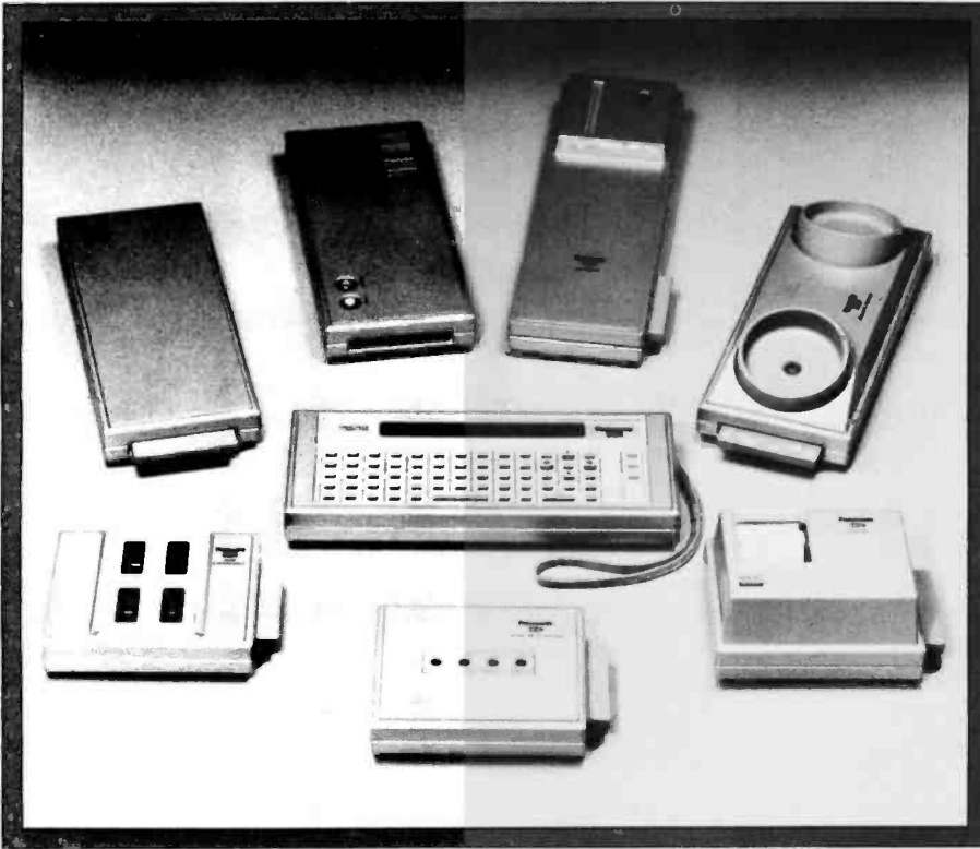
Photo 2: The HHC and its peripherals. The HHC computer is in the center of the photograph. The peripherals are (clockwise, from upper left): a programmable-memory extender, the color television interface, the I/O driver (a distributor of bus signals from the HHC to other peripherals), an acoustic-coupler modem, a portable printer, a cassette interface, and a ROM expander.
