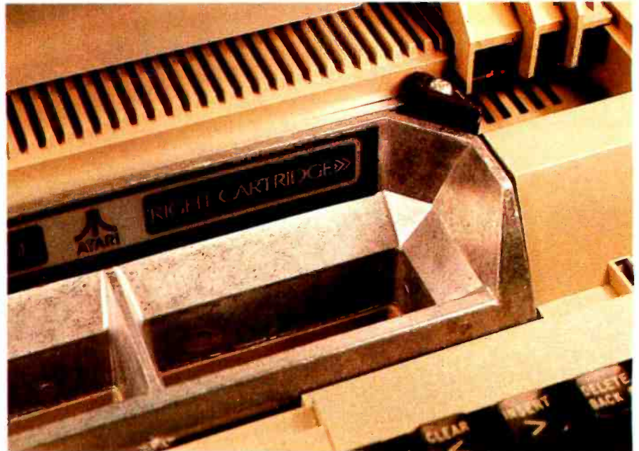
Photo 7: The Atari computers allow the user to plug in special game and business program cartridges. These ROM packs (read-only-memory modules), which are connected directly to the processor bus, must also be kept within the shield when the computer is running. This is accomplished using a special molded, 3/8-inch (9.5 mm)-thick socket that is electrically part of the shield. A plate of aluminum with conductive gasket material around the edges is attached to the cover. When the cover is closed, the memory is completely shielded and virtually no electrical noise is emitted.
