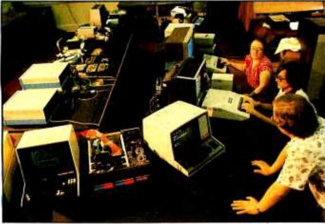
Photo 2: The equipment currently available in the Solo/NET/works laboratory. The terminal at the lower left in Photo 2a is used for the WAG display (as explained in the text). To its right is the IMSAI 5-100 computer that emulates the unrooted-tree network and performs the managerial WAG functions. Further to the right are the system console and bus-status monitor; the other microprocessors operate as nodes in the network. Photo 2b shows MATSRCH designer Ivan Zatkovitch using an Apple II computer in a version of the game that requires only one player.
