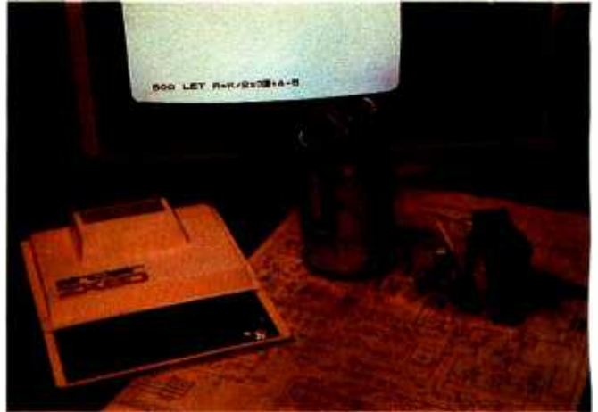
Photo 1: A photograph of the ZX80 in operation. The homemade power supply gives an indication of the small size of the computer. At the bottom of the television set, a BASIC line is being edited.
