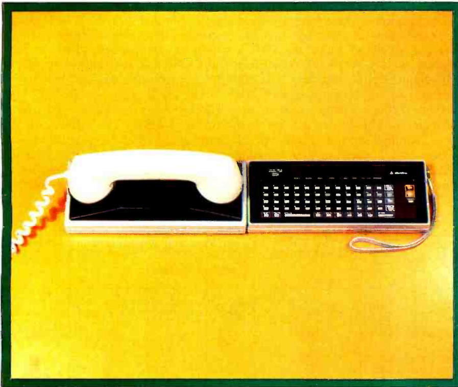
Photo 4: The Quasar HHC connected directly to its acoustic coupler. The combination, which is also available in the Panasonic HHC system, is a self-contained portable computer terminal.
