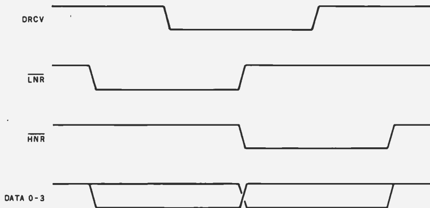
Figure 2: Timing diagram for information transfer using the cable scheme of figure 1. The transmitting computer puts information on the DATA lines, low-order nybble first, and brings the LNR line low. The receiving computer brings the DRCV line low when the information has been accepted. The process is repeated for the high-order nybble, but HNR is used to indicate the presence of new data. When DRCV is brought high, the transmitter and receiver functions reverse.
