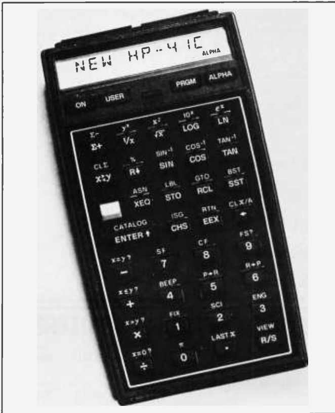
Photo 1: The Hewlett-Packard HP-41C calculator. Each key on the HP-41C has up to three labels associated with it: the label etched into the top face of the key, the label visible directly above the key, and a letter of the alphabet (enabled by toggling the ALPHA button) etched into the bottom face of the key. Additional functions are called by hitting the XEQ button and spelling out the function name. (Photo courtesy of Hewlett-Packard.)
