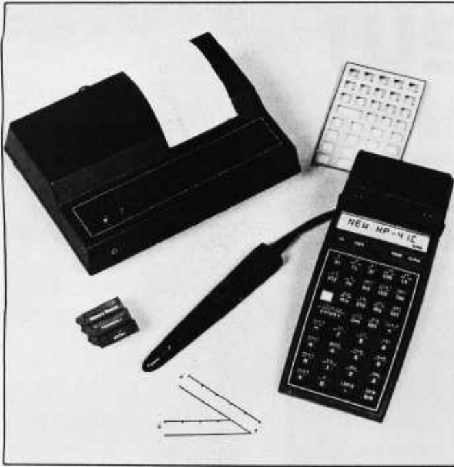
Photo 2: The HP-41C and accessories. Clockwise from top are: the 82143A peripheral printer, a key overlay (for use when redefining key functions), the HP-41C with the 82104A plug-in card reader, two magnetic cards, and three read-only-memory application packs. In the center is the 82153A bar-code wand, which is used to read software printed in the form of bar codes. (Photo courtesy of Hewlett-Packard.)
