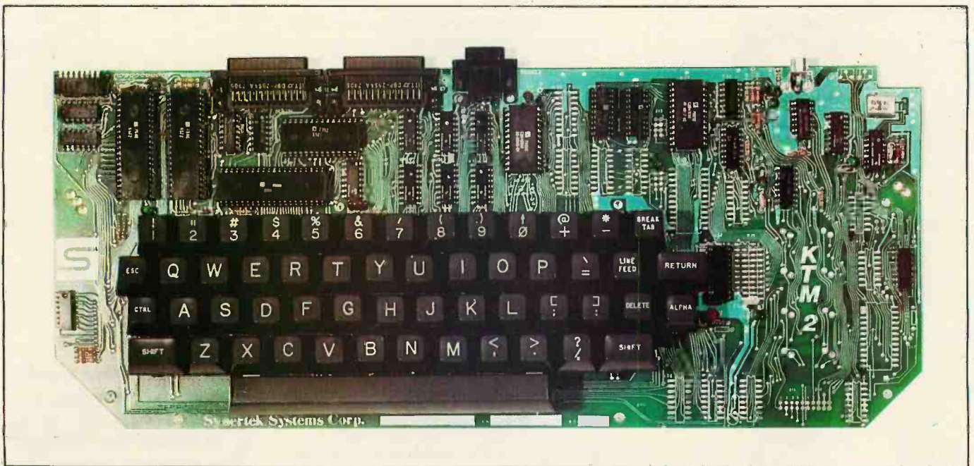
Photo 1: The KTM-2 board. The board contains a 54-key array, with all the circuitry necessary for composite-video output. This 40-character per-line version requires 1.4 A at 5 V. The 80-character version draws 1.6 A. Both are able to provide RS-232-compatible outputs with the addition of extra power supplies.
