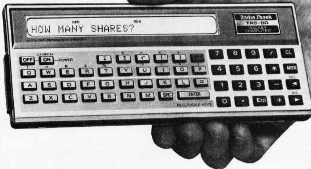
Photo 3: The TRS-80 Pocket Computer. Measuring 17.78 by 7 by 1.27 cm (7 by 2¾ by ½ inches), the hand-held unit sells for $249 and can be programmed in Level I BASIC. The display is 24-character liquid-crystal type utilizing a 5-by-7 dot matrix. There are 1.9 K bytes of programmable memory included, and a cassette interface (list price $49) is available for off-line storage. Eight software packages are currently available, including Aviation, Real Estate, Engineering, Finance, Games, and Math.
