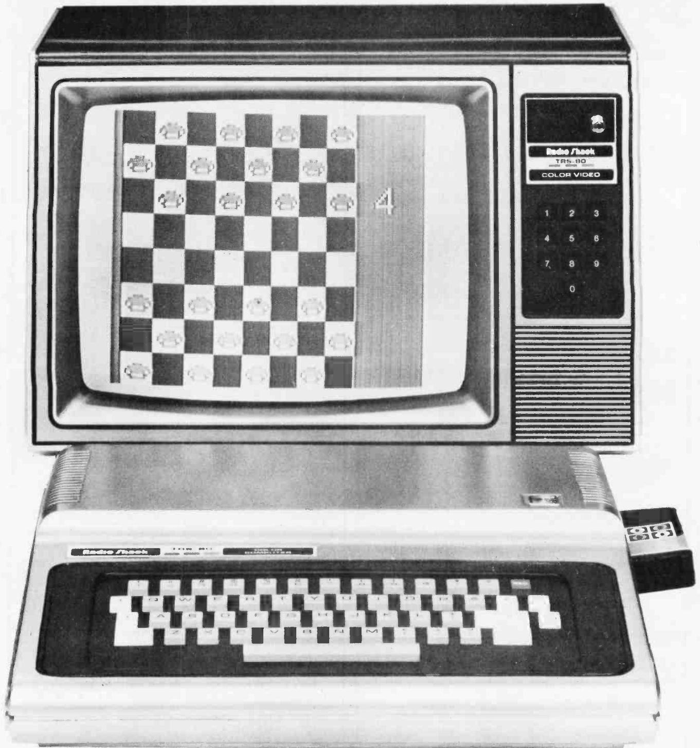
Photo 2: The TRS-80 Color Computer sells for $399 with BASIC, 4 K bytes of user memory, and a built-in television RF modulator. It supports eight colors and several levels of graphics resolution. Eight game programs are currently available on ROM-based "Program Paks" that plug into the right side of the unit. Expansion is available with 16 K of programmable memory and Extended Color BASIC, which allows the creation of high-resolution graphics from within a BASIC program. The monitor shown receives standard television signals and sells for $399.
