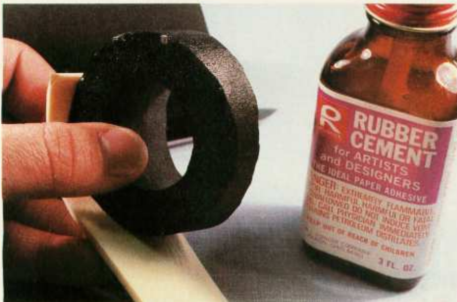
Photo 5: Adding pliable material to produce a tight fit around the phone handset. I found a plastic placemat at a discount store with a 1/4-inch foam backing that was perfect. Cut a strip 1 1/2 by 8 inches and glue this around the outside of the wedge as shown. Trim to the exact circumference and cover with a strip of fabric adhesive tape. The latter helps hold everything together.
