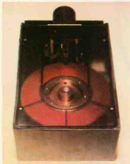
Photo 4: BASF Systems' 6170 Series 8-inch, fixed hard-disk drive, available in 8- and 24-megabyte versions. (Photo courtesy of BASF.)
