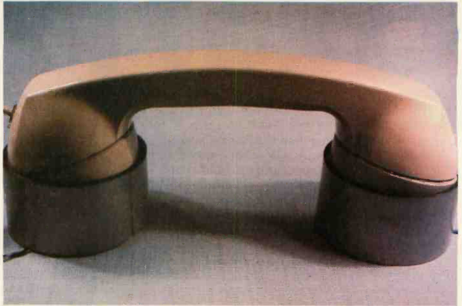
Photo 9: With the production of two of the speaker assemblies I have described, we are in business. The one wired to the microphone input of the modem should be placed under the earpiece of the phone, and the one designated as the modem output speaker against the telephone mouthpiece. Dial your favorite computer, place the handset in the coupler, and when you see the carrier-detect indicator light, you are ready to go.
