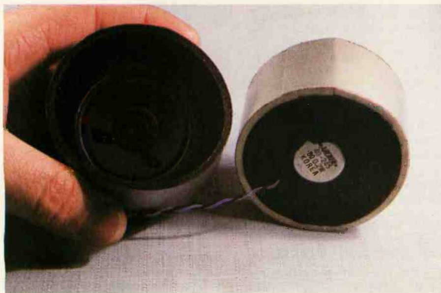
Photo 6: Insert the speaker into the hole and align it with the angle of the foam wedge. In the unit shown, I used a black broad-tip marker to darken the white surfaces on the inside.
