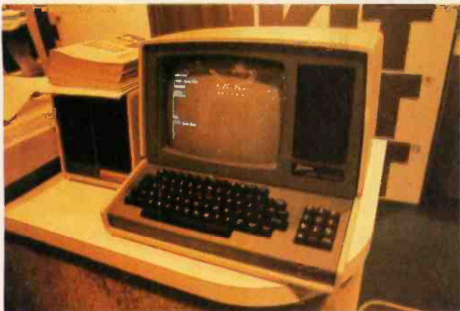
Photo 1: The Heath H-89, a Z80-based all-in-one personal computer with built-in 5-inch floppy-disk drive, WH-19 terminal, and 16 K bytes of programmable memory (expandable to 48 K bytes). The price for the assembled unit is $2295.
