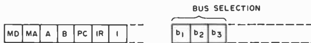
Figure 4: Portion of a horizontal microinstruction to control the connection of registers to the bus in figure 3. Each box is a microinstruction bit that enables the indicated register-to-bus connection.
