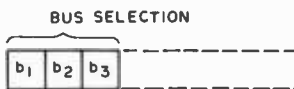
Figure 5: Portion of a vertical microinstruction to control the connection of registers to the bus in figure 3. Here, three bits are used to encode a choice between seven registers or a 0 "no operation."
