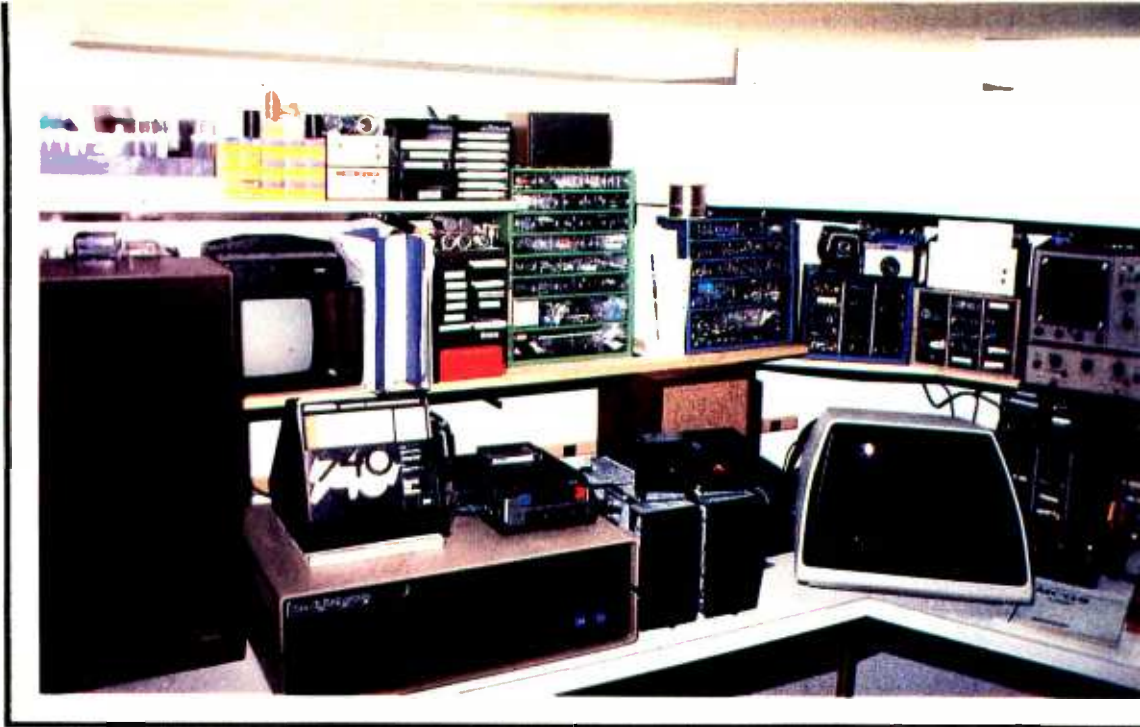
Photo 3: Corner of the circuit cellar showing the 64 K dual floppy disk Z-80 system used by the author to drive the musical tone game.
