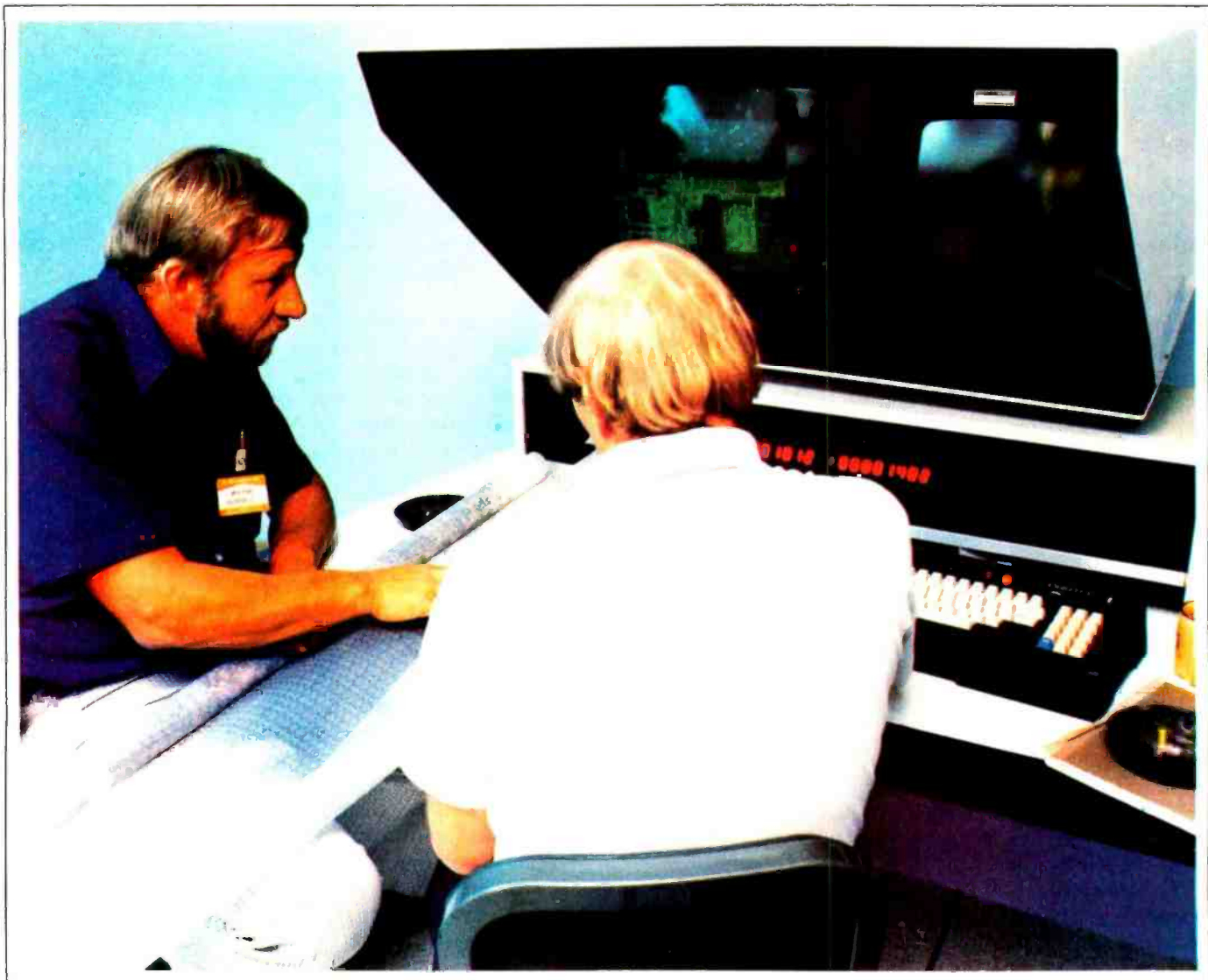
Photo 4: Editing the layout. Drafting manager Wayne Busfield and senior layout designer Rick Secrist make changes indicated by engineering analysis. This iterative process improves performance and production yield, and thus lowers cost.
