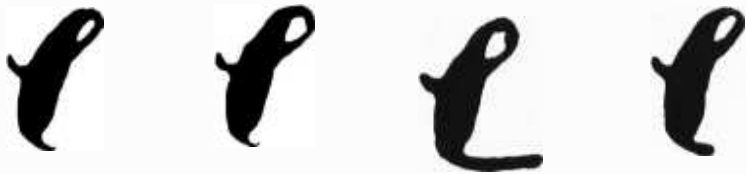
Photo 1: Four successive es drawn by the Maillardet machine, showing the consistency of the mechanical drive system as well as the variations in letter width that were possible using a quill pen.
