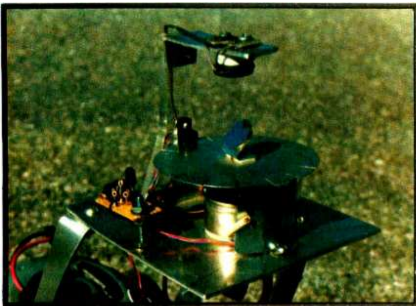
Photo 1: The primary sensor of Tee Toddler is this photoelectric horizon scanner. The "eye" mounted on a Plexiglas standard and metal bracket scans a 360° field. The flat mirror rotates at five revolutions per second deflecting light into the phototransistor eye through a 45° angle. The position of the mirror is resolved into one of 16 angular states by a slotted disk which passes through an optocoupler.
