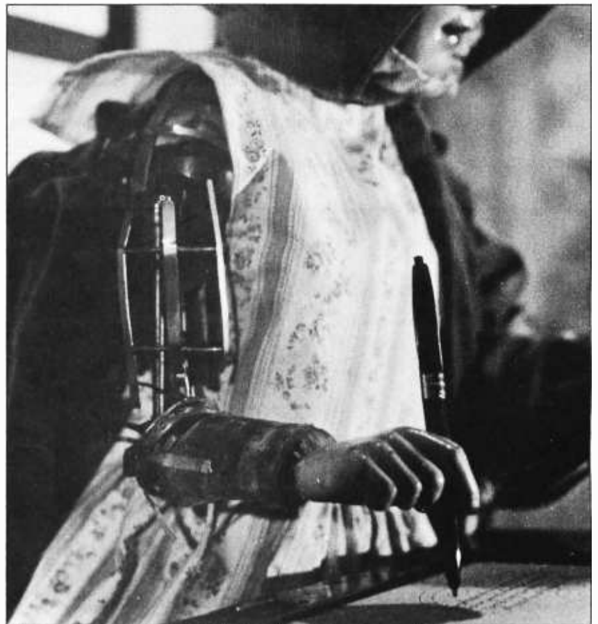
Photo 2: Right arm of the automaton, undraped. Modern ballpoint pen is not historically correct, but is effective.
