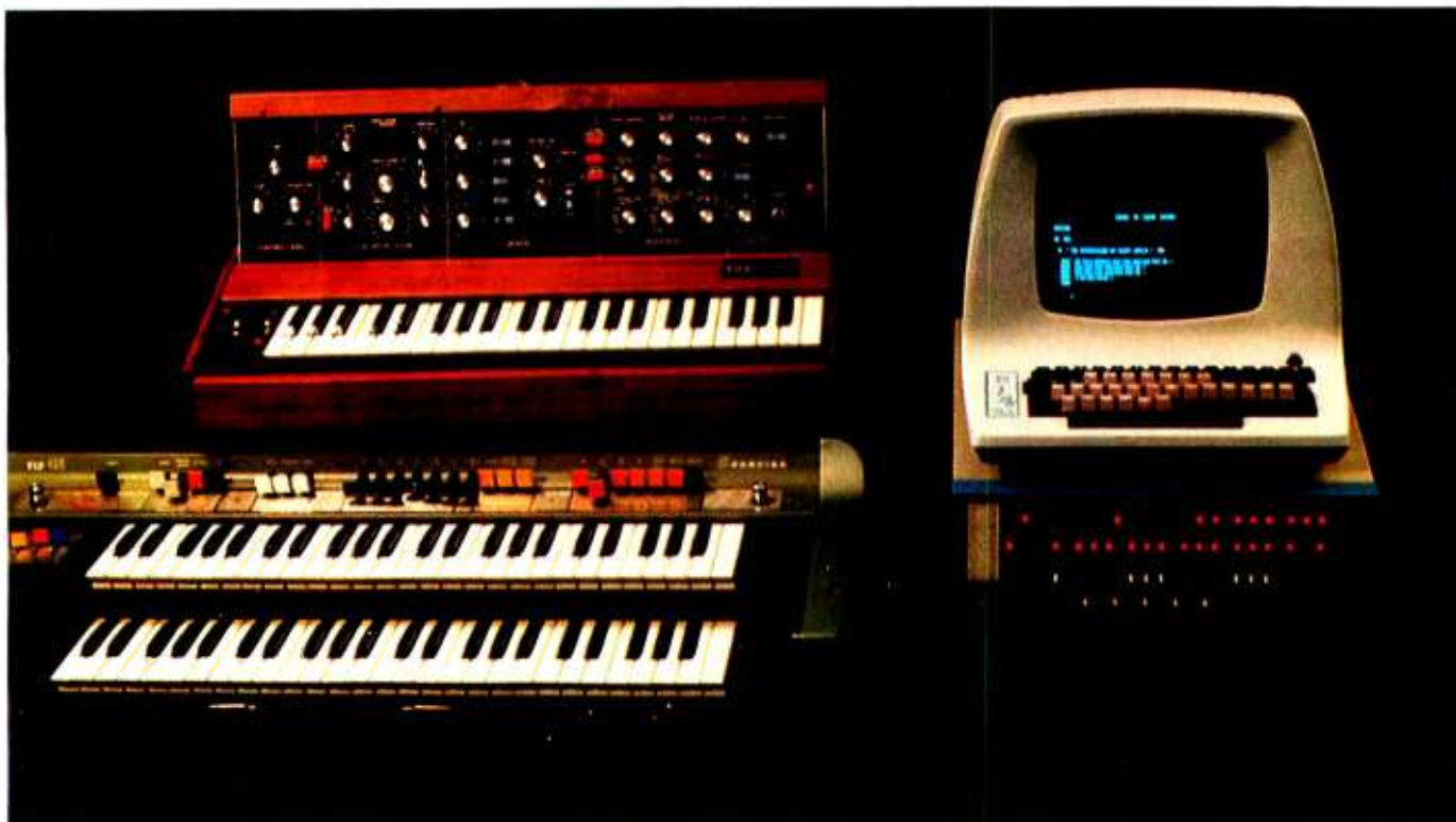
Photo 1: The author's computer music system, which consists of an Altair 8800 computer with 32 K bytes of programmable and read only memory, and an ADM-III video terminal. Also pictured is a Mini-Moog electronic music synthesizer (top left) and a Farfisa VIP 400 electronic organ (bottom left).
