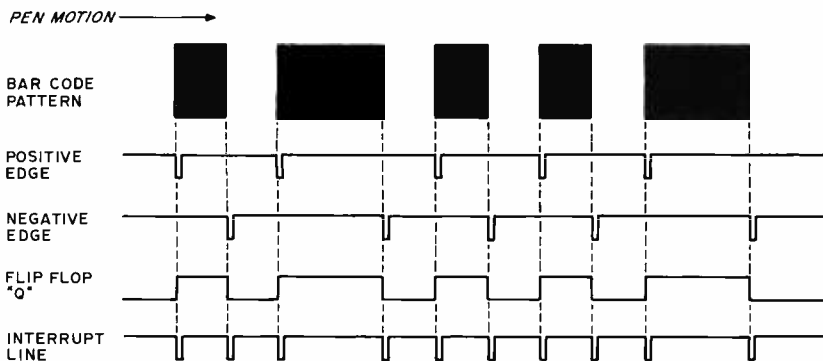
Figure 4: A "Super Differentiator" Signal Conditioning Circuit. This circuit is edge sensitive and outputs short pulses at each black to white or white to black transition. The timing diagram shows the outputs of the circuit, corresponding to the bar code pattern shown.
