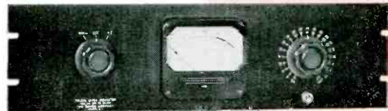
Type 915 Rack model, terminating and bridging type. Meter multiplier ranges: Terminating, —6 VU to +32 VU; bridging +4 VU to —42 VU; or terminating, —6 VU to +16 VU; bridging, +4 VU to +26 VU. 2 VU steps. Reference level: 1 mv into 600 ohms.
