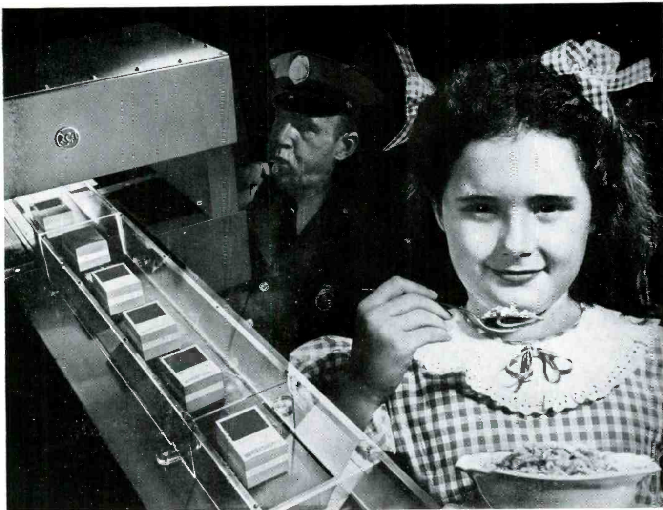
The RCA Metal Detector "blows the whistle" on any particle of metal that may have crept into the package.
