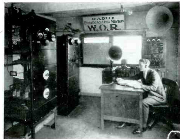
500 Watt Transmitter on the roof of L. Bamberger & Co., Newark, N. J. 1922.
