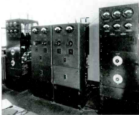
October, 1922, 24 Walker Street, New York City. WBAY's (now WEAF) first radio transmitter.
