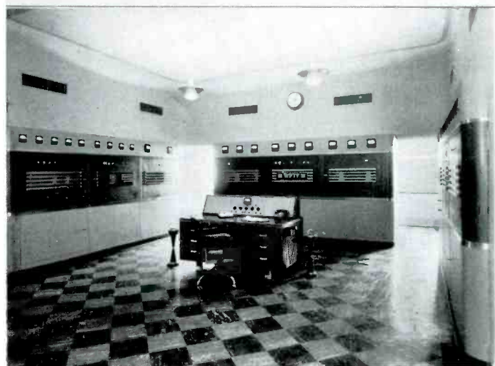
Interior of transmitter building showing new Westinghouse 50-HG transmitter
