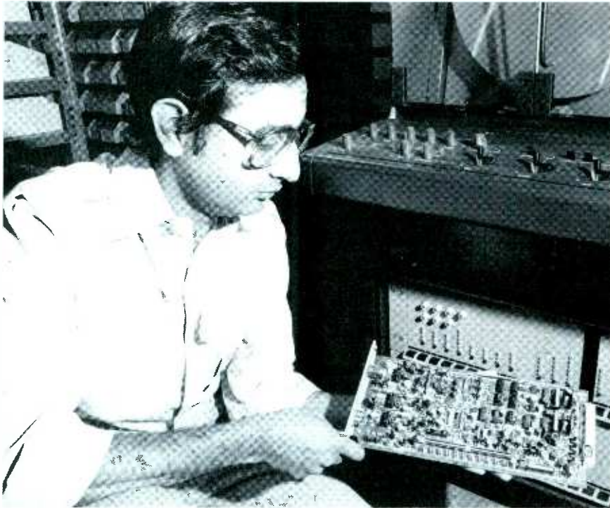
Fernseh engineering services manager K. Jayaraman shows one of the boards (a servo controller) from the FDL 60.
