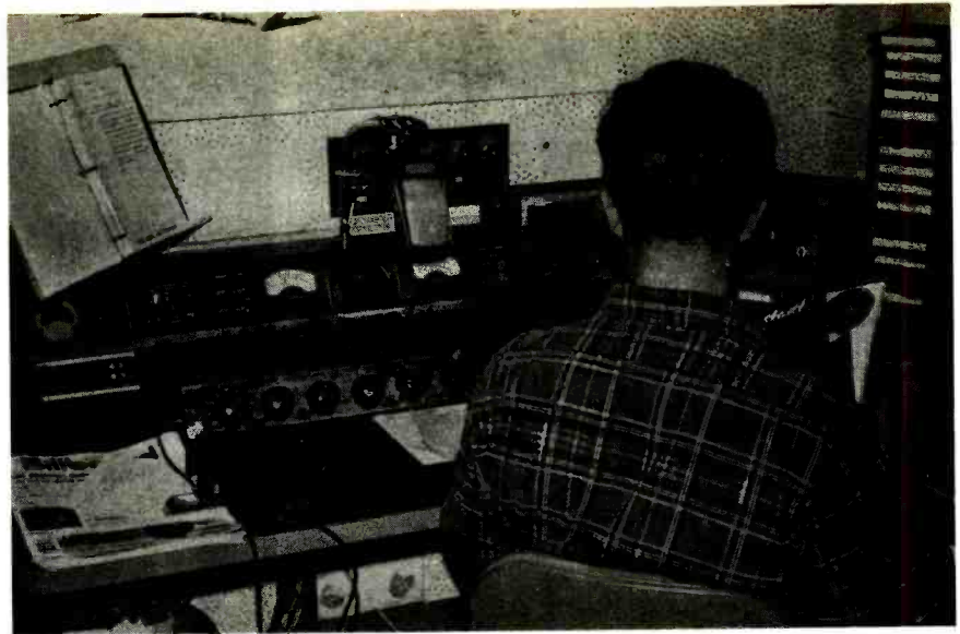
KAWC master control. The Western Electric console actually has all-new solid-state plug-in module electronics.
