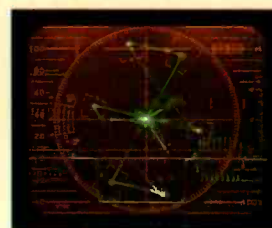
Combination Display— Simultaneous waveform and vector displays of a single input
