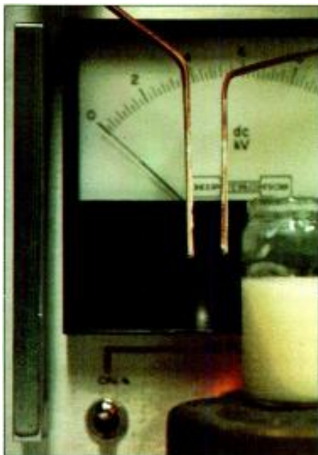
Recently developed electro-rheological fluid adjacent to electrodes used to create electric field for solidifying the fluid.
