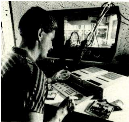
The Philips LHH 2000 CD player system uses a flywheel for cueing.
