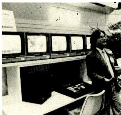
Convergence's new ECS-1000 is a self-contained editor with 1000-line EDL.
