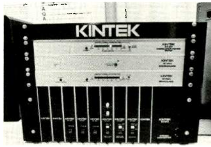
The new Kintek KT-960 Monoguard prevents loss of mono due to polarity reversal for MTS.
