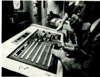
Intergroup Video Systems introduced the 9420 20-input production switcher.
