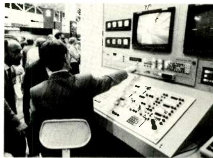
Grass Valley Group's Model 300 had a versatile new key extender.
