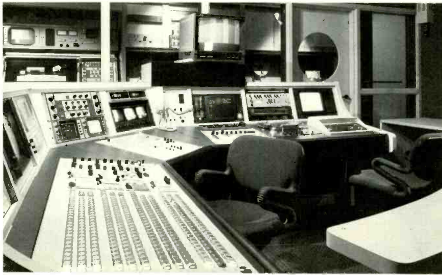
Edit room one features a Grass Valley 300 switcher, a CMX 340X editor, a Grass Valley Mark II DVE, and Ampex VPR-3 tape machines.
