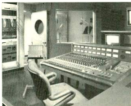
Editel's audio room features an MCI/Sony 618 console, an MCI/Sony JH-24, and a Mitsubishi digital two-track.
