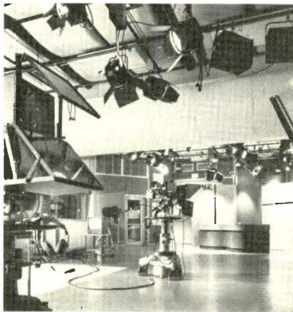
The 40x60-foot studio has Hitachi SK-70s, Ikegami 302s, and Strand Century lighting.
