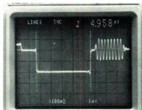
The \Delta_V and \Delta_t cursors of the 2400 Series scopes with TV Option provide a convenient, accurate means of verifying waveform timing and amplitude parameters.
