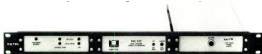
The cable audio scrambling system from Catel.
