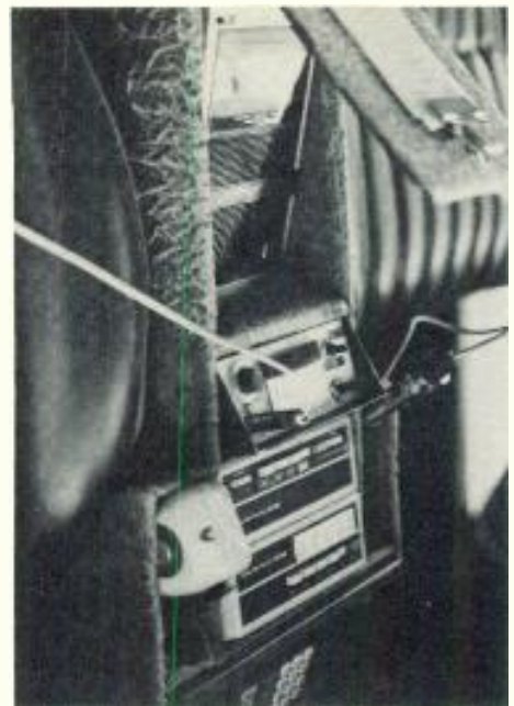
Mobile equipment plays cassette sound as part of live report; from left, cassette deck, control head, Motorola control.
