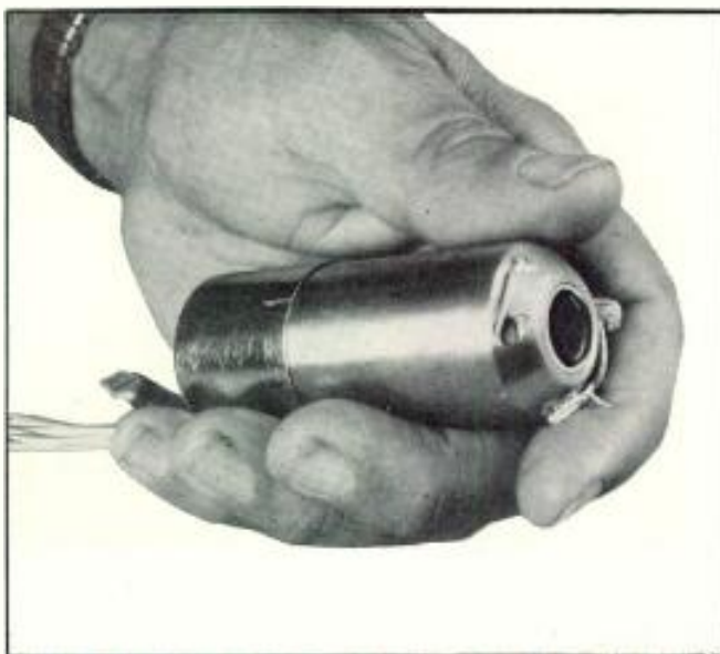
A new deflection coil design in the RCA-developed tube requires no additional clamps or hardware.
