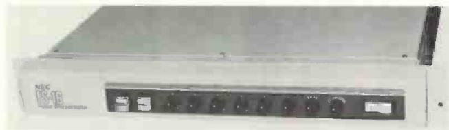
NEC's FS-16 offers proc-amp functions and frame synchronization.
