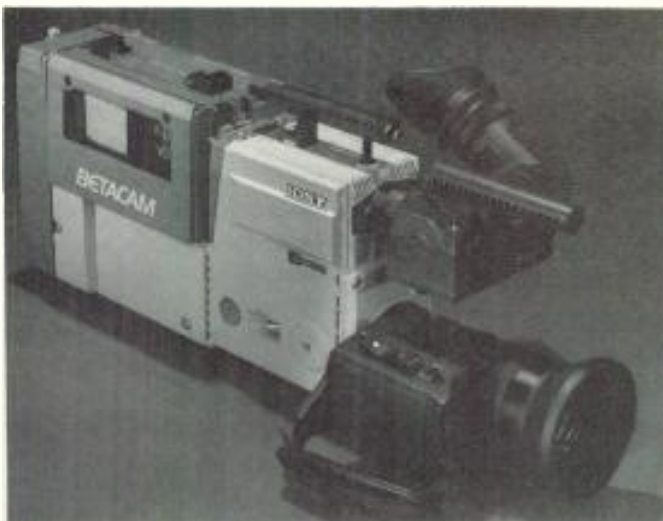
The recorder on Sony's Betacam is now detachable.
