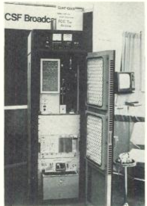
Thomson-CSF brought the only LPTV transmitter actually on display. The LGT EUHF-1000S all solid state 1 kW UHF model, FCC-type-accepted, was described by a spokesperson as "the Rolls-Royce of low-power transmitters."
