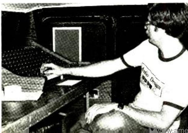
Operator inside van has mixing console for the 15 microphones used in the pickup. He had intercom to band leader, monitor circuits for all pickups
