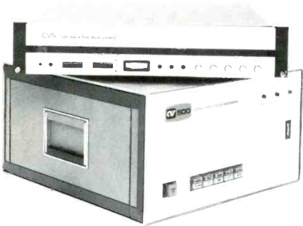
Dramatic size reduction of TBCs is demonstrated by the difference between CVS' first TBC, vintage '73, and its Model 520, vintage '76.
