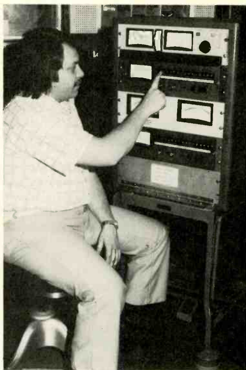
Here disc jockey Bradford Baad operates Remote Control Panel. The equipment sets atop a very sturdy metal typing stand. Casters on stand allow the equipment to be easily moved. All lines to and from the control panel are formed into a long umbilical cord which permits moving from studio to studio.
