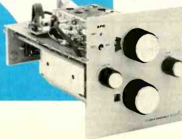
VT-4B-1 Plug-in Variable VHF/UHF Tuner
