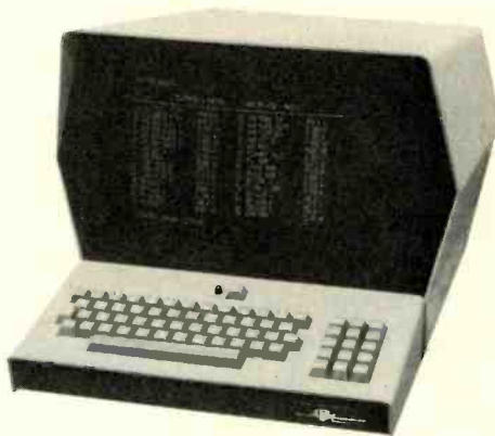
Fig. 8 CRT display used with computer-assisted remote control system enables the simultaneous presentation of 30 metering or status functions. All command functions are entered through keyboard.
