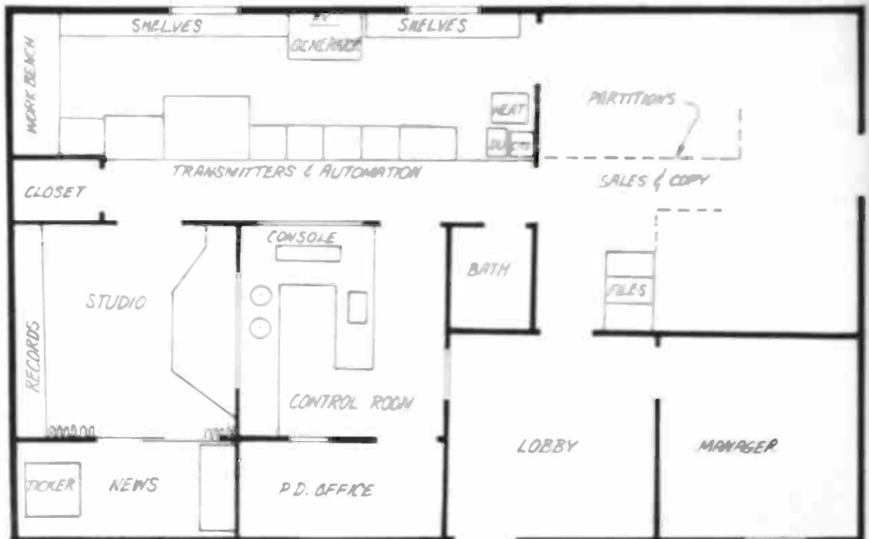
From the control room of this compact layout at WOOD, the operator can see the studio, the news room, the automation gear across the hall, and even the secretary in the lobby.
