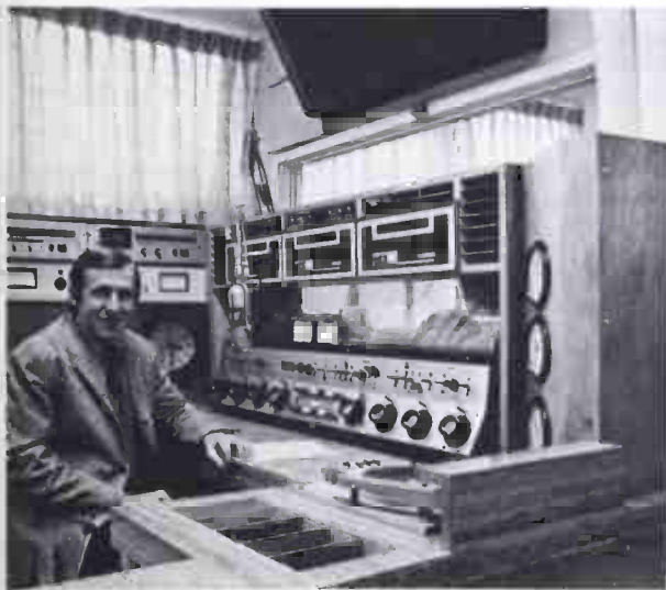
Ed Marks in the new Master Control Room. That's a window below cart lines (Gates) and above the control board (Gates President) looking into Production Studio A. Behind program director Ed Marks, are remote control panels and monitors for AM and FM operations. To the left is a window in FM automation room.
