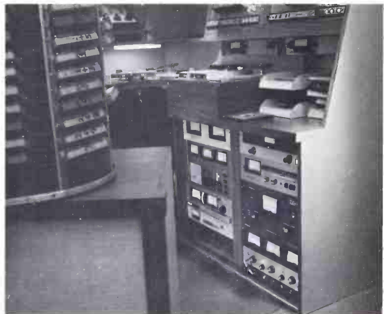
Control Console for the remote control of the AM and FM transmitter.
