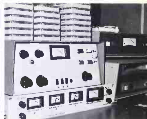
Close-up of recording facilities: Gates Criteria 80 cart record/playback unit, Dorrough Model 313 audio processor, KVOO designed audio control and digital timing/encoding system. Gates CB77 turntables not shown.
