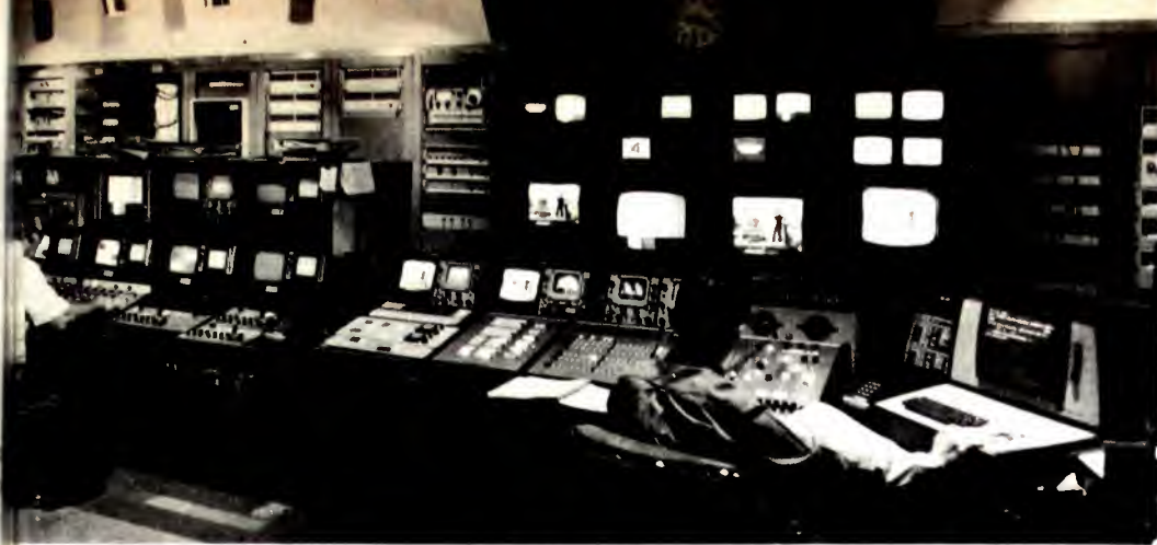
Master control room at KYW-TV. CRT terminal input to automated switching equipment as at far right. Between it and switcher is video monitor displaying upcoming events.
