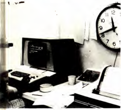
Girl in Traffic entering the program schedule into automated switcher computer. This step will be eliminated shortly; central computer will feed data directly to switching computer.
