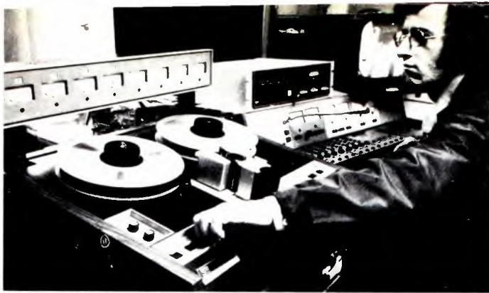
Sound mixer adjusting control on the 3M series 79 recorder. The Synchronizer/Reader unit is on top of the Philips audio mixing console.
