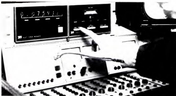
Close-up of the Synchronizer/Reader which provides the capability of synchronizing audio with video.
