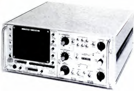
Model 711/801B spectrum analyzer combines storage display unit with analyzer tracking BFO. Other models combine basic units in other pairings.
