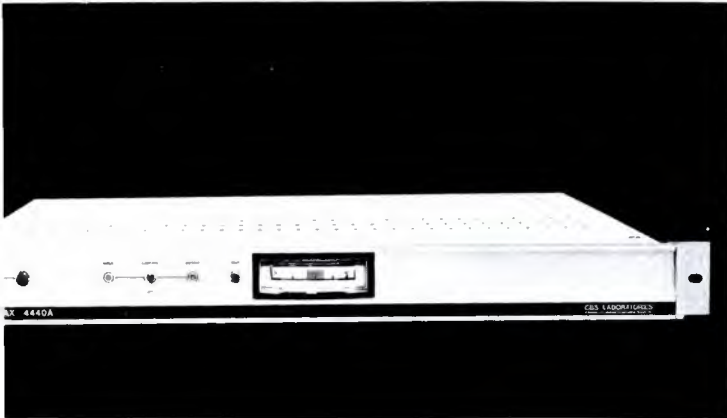
CBS Audimax is a compressor with a "gain platform" that reduces noise "pumping" in signal pauses; the gain is held constant during short pauses.
