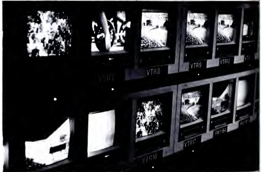
Monitor wall showing part of the monitors used to indicate VTR feed in the VTR control room. Up to 13 simultaneous programs could be handled.
