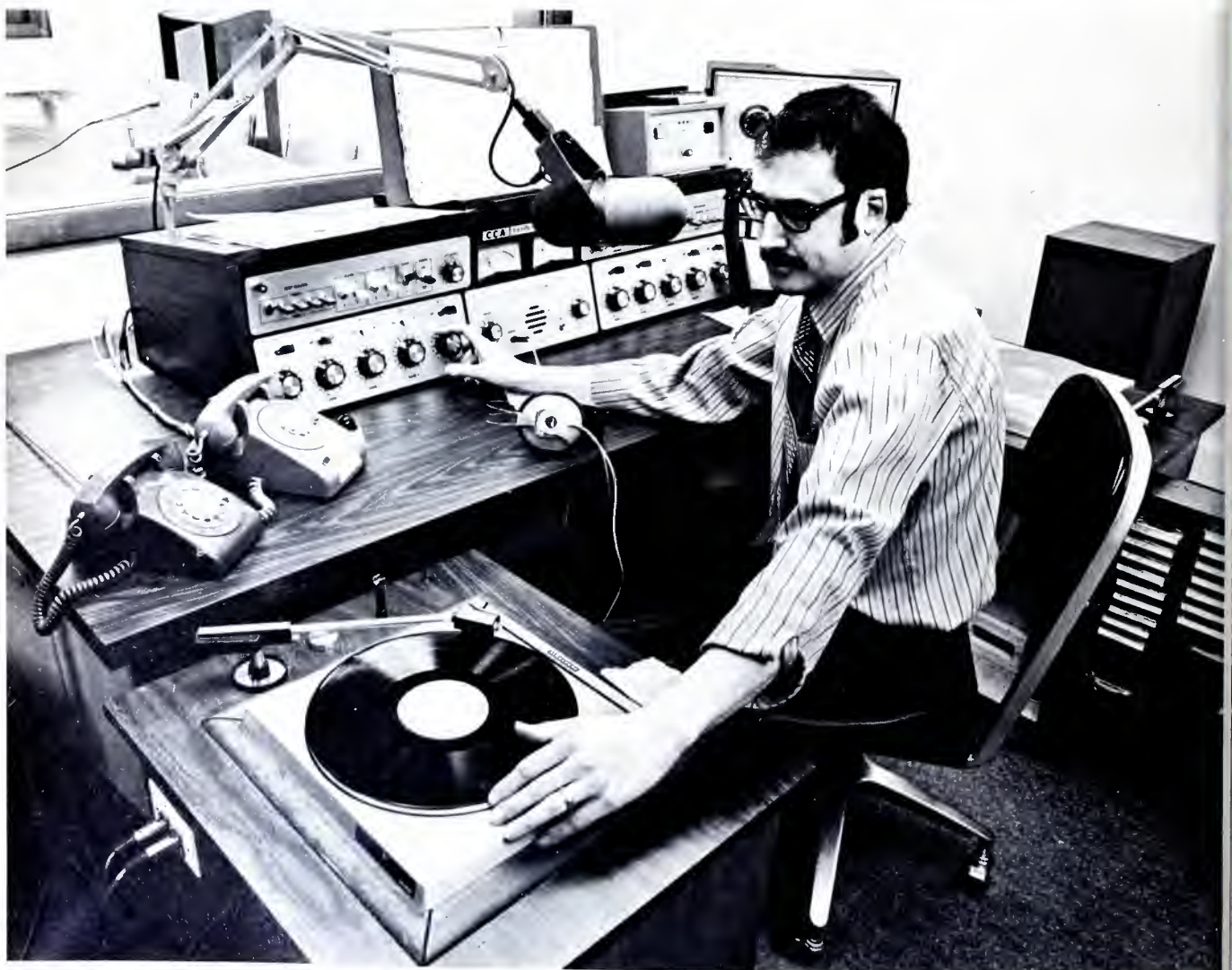
WYEN says the SP-10 turntable replaced a more expensive professional unit which exhibited excessive rumble even after motors were reworked.
