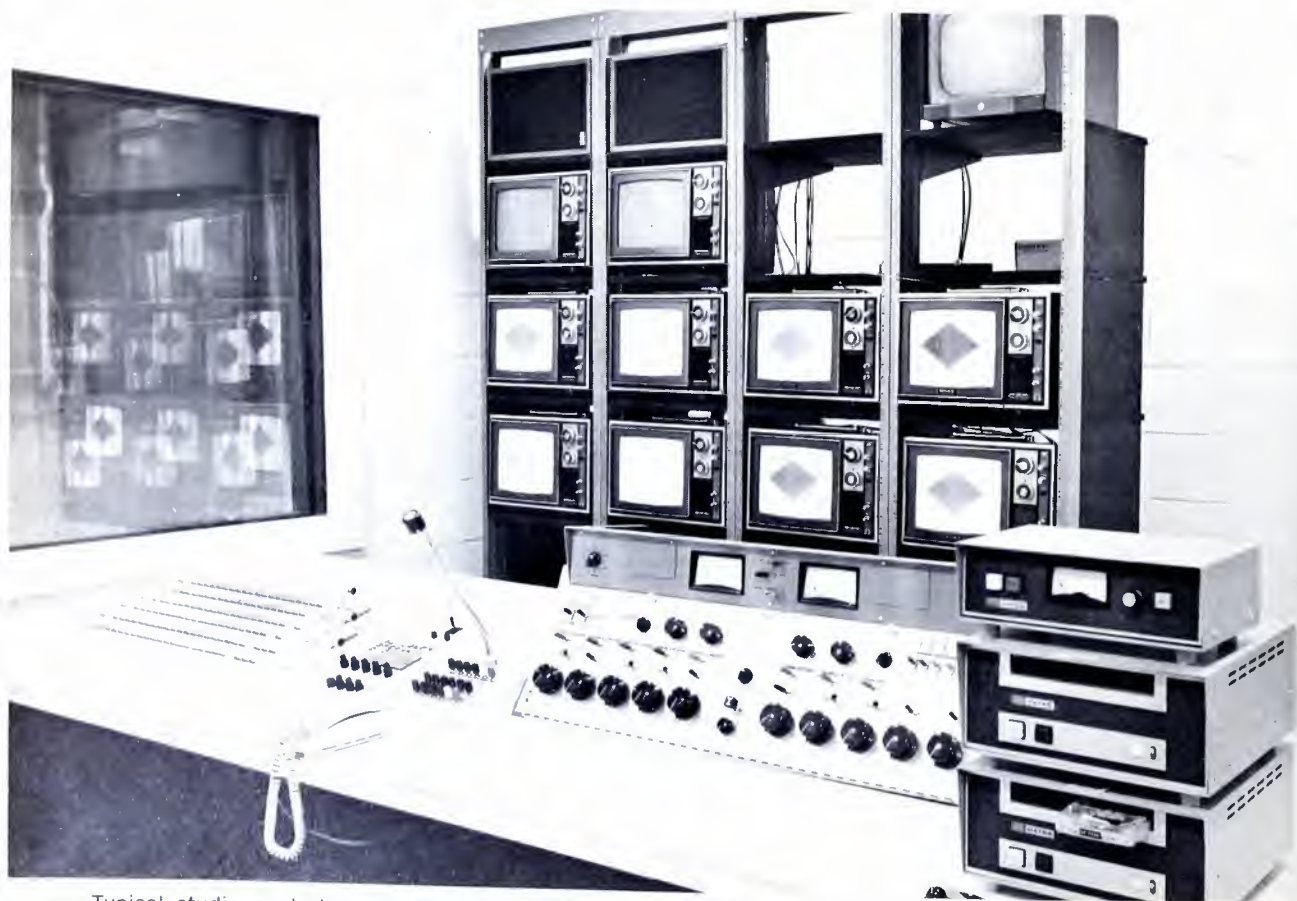
Typical studio control room showing new Grass Valley switcher, RCA audio console, and Gates cartridge tape equipment. Monitors are "jeeped" Sony 1201 color receivers.
