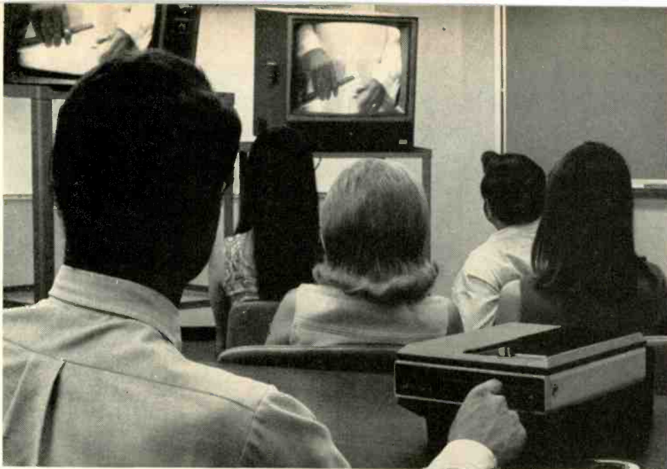
Smallest cartridge-loading video recorder to date is Ampex Instavision player, in foreground.
