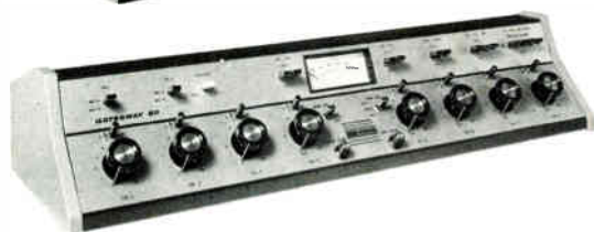
Gateway 80 audio console: 18 inputs into 8 monaural mixing channels; modular solid-state amplifiers, step-type attenuators.
