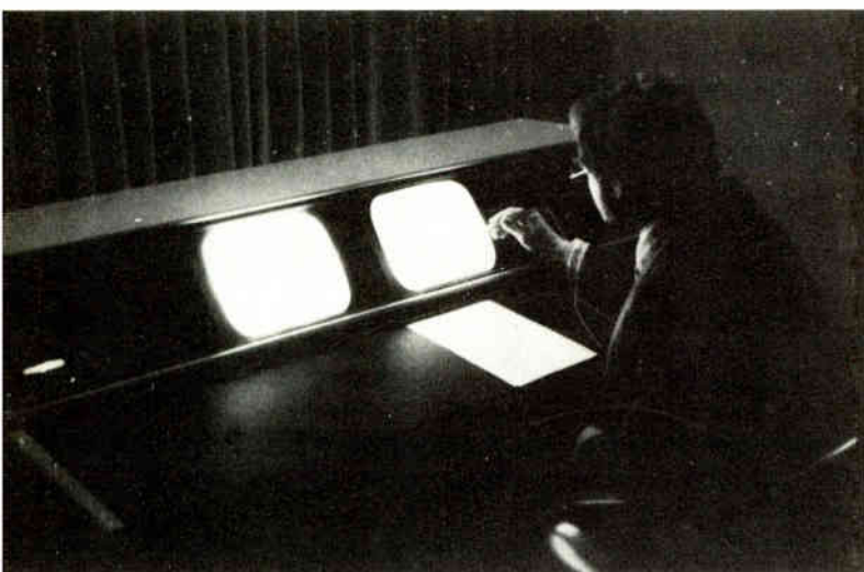
Use of videotape in original shooting of motion pictures and advertisements is being greatly encouraged by a flock of new, highly efficient videotape editing systems. With one of the most highly automated, the CMX system, the editor merely applies a light pencil to screen (above) to "tell" the system what he wants— follow-through is automatic.
