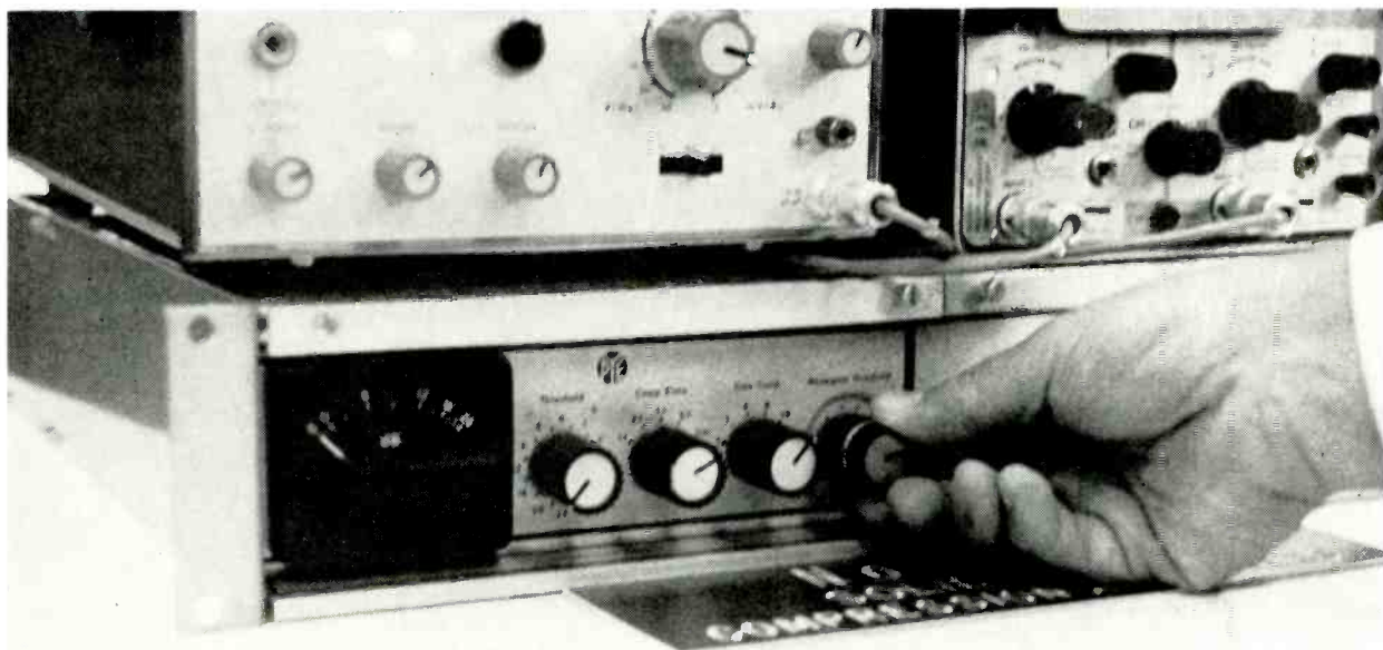
Compression amplifier type 5752 and 5753 from Norelco/Pye, uses pulse modulation.
