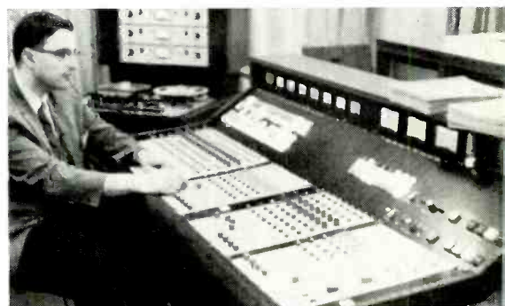
Three-in-one Weigand console has 14 inputs for 8-track recording. Unit also has remix capability.
