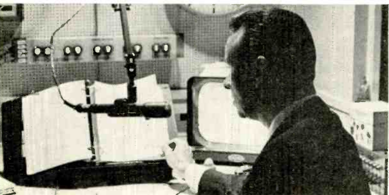
Announce studio next to Master Control contains video monitor and repeater of Visual numerical readout as it appears in control room.
