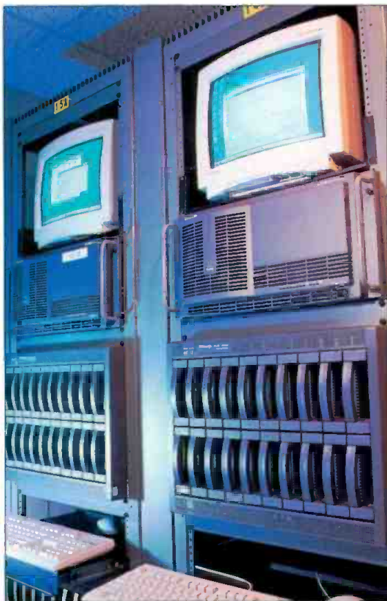
Dual PDR204D Profiles with mirrored storage provide more than 50 hours of storage.
