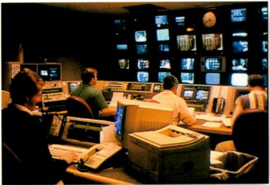
The networked control room will allow WXYZ staff to direct the on-air playback of both HD and multichannel using Omnibus networking and Profile servers.
