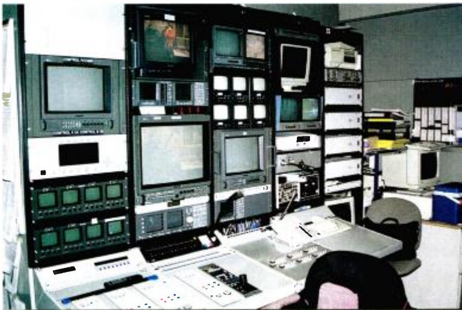
The videotape and CCU at KTVT. The Telex Adam "list" function allows users to be assigned group communications as needed, preventing everyone from having to hear all communications.
