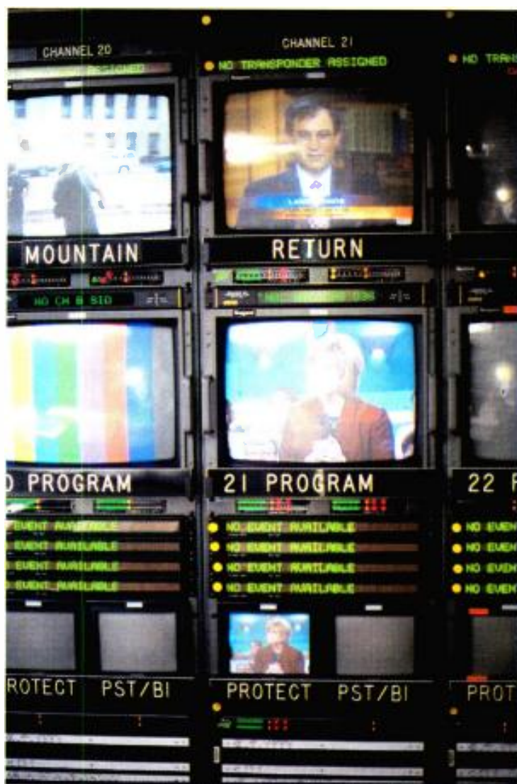
Six channels of surround sound audio and multiple video channels require new space-saving methods of audio metering. Shown here are Logitek under-monitor VU meters.
