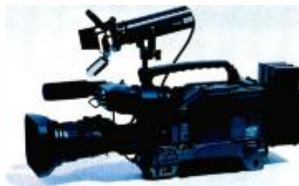
Frezzi Sun Gun HMI on Sony AX, all powered by hot swap NP1-3P1 with Frezzi FND-1MH battery.
