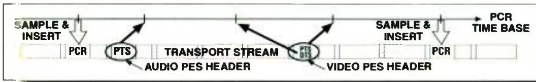
Figure 3. A single-program transport stream showing PCRs and time stamps, essential for timing and synchronization.
