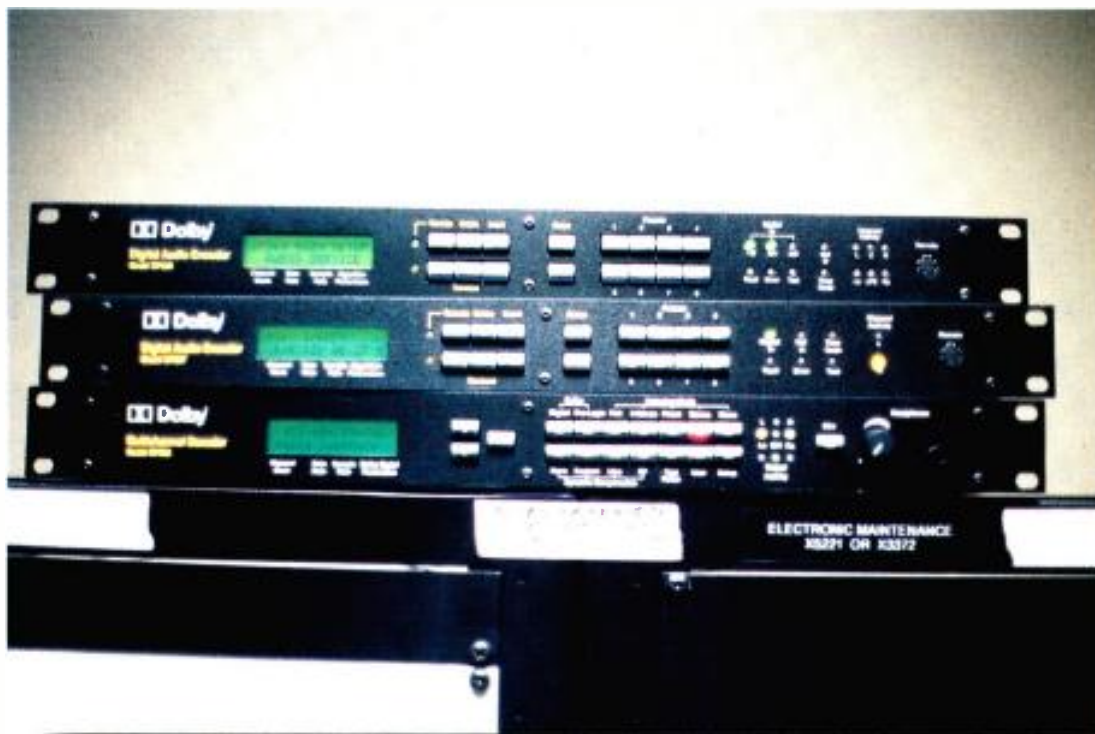
Many stations will want to purchase audio encoders so they can produce their own surround sound. Shown here are the Dolby broadcast encoders.
