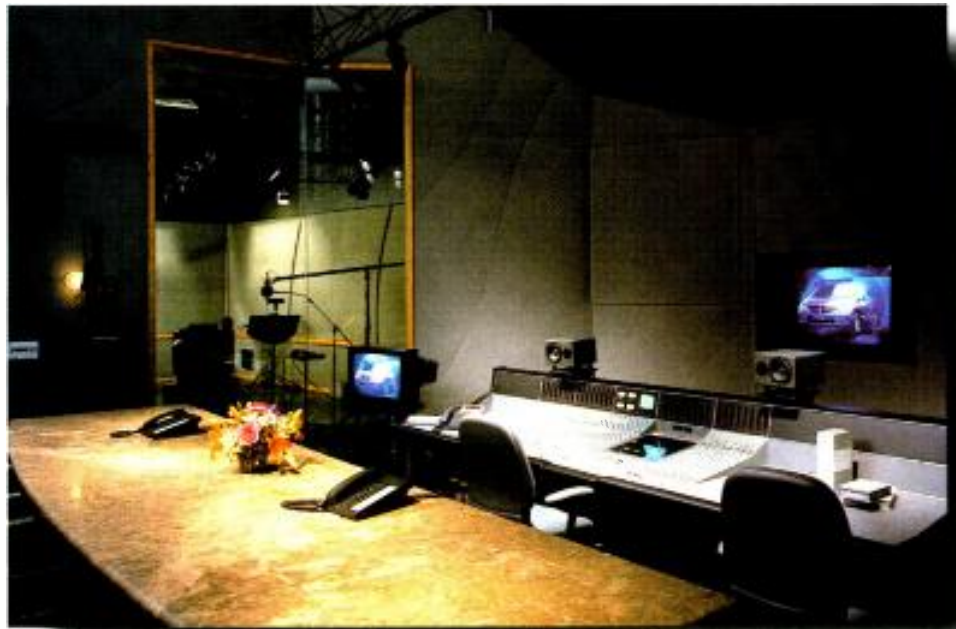
GTN, Detroit, MI, an audio/video production and post house installed two Solid State Logic Aysis digital 64-channel mixing systems to provide 5.1 surround-sound mixing capability. The new equipment affords users 144 hours of shared storage in combination with the facility’s networked SSL DiskTrack and ScreenSound digital editor and VisionTrack.
