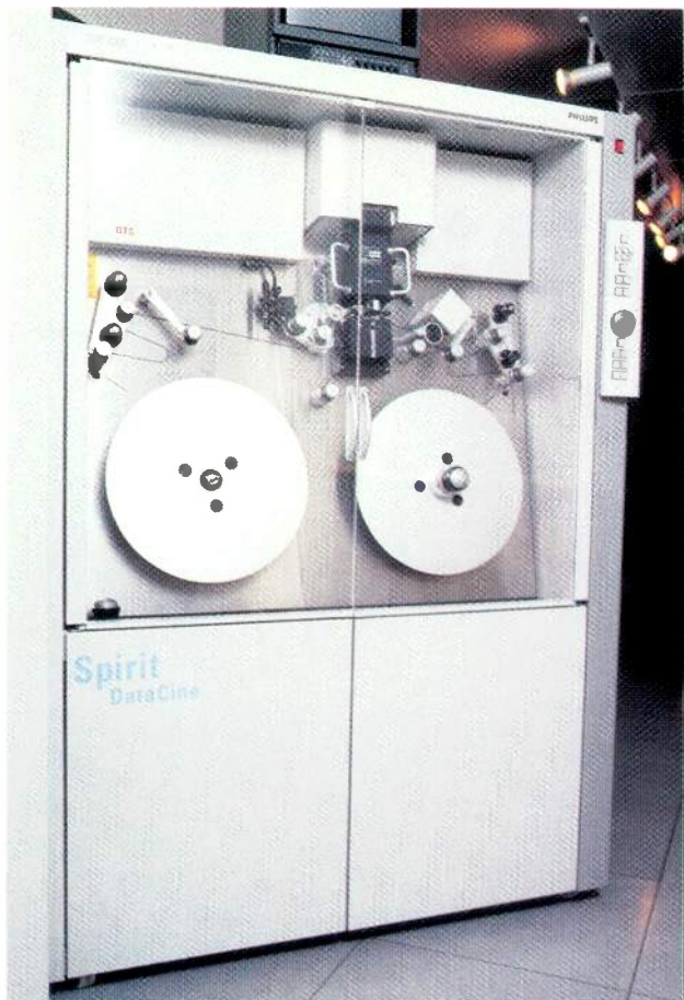
The Philips Spirit DataCine was recently upgraded so it can output in real-time 4:4:4:4 resolution via an HIPPI interface at 600Mb/s.
