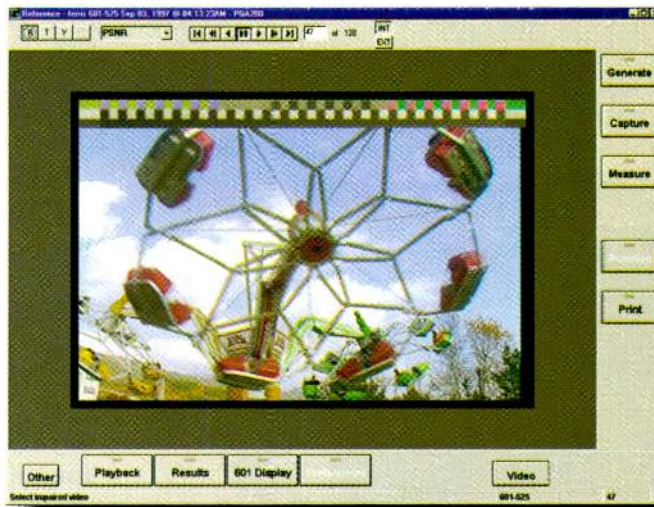
Figure 2. The calibration stripe on the first two seconds of each sequence reduce the processing power (and time) needed to perform subpixel alignment of the degraded and reference scenes. The stripes also contain segments for chroma and luma changes and frame ID for temporal alignment.
