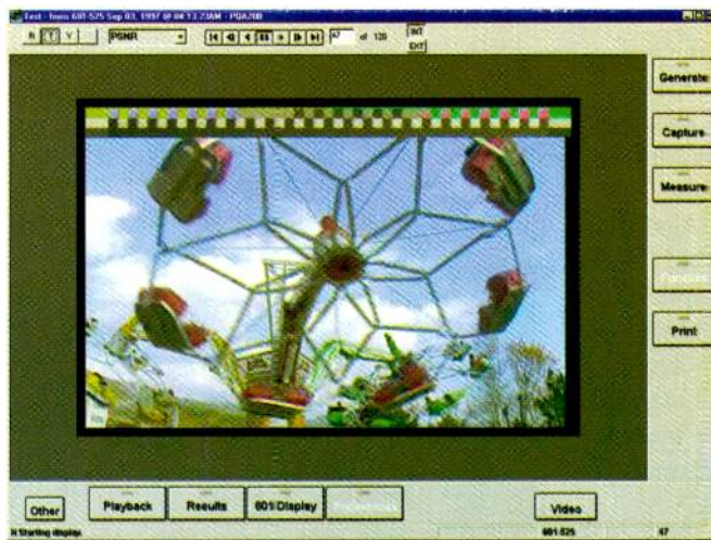
Figure 3. This single-frame degraded image shows a significant loss of detail in the lower right corner and considerable blurring of the spinning wheels of the ride. However, the fact that the wheels are in motion reduces the perceptibility of those distortions — as can be seen in the PQR map. (See Figure 5.)
