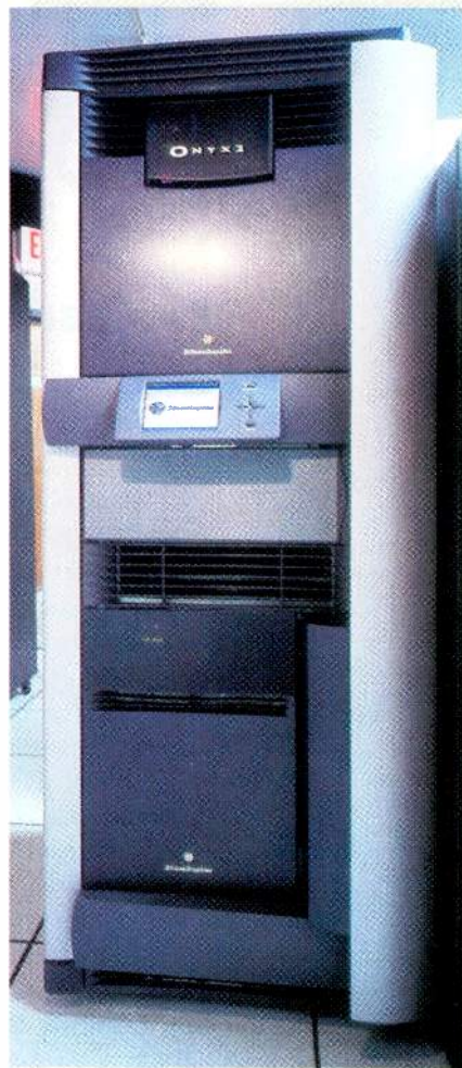
Crawford's SGI Onyx 2 was recently used to demonstrate film-to-HDTV translation into the computer over an HIPPI network at 6fps.
