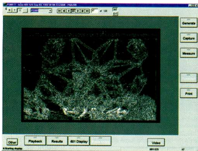
Figure 4. The PSNR map is a relatively raw picture difference display, indicating the pixels most different from the original with the brightest luminance levels. Notice that it does point out the changes in the bottom quarter of the display and the loss of detail in the lower right corner. However, the PSNR map also shows significant changes in the wheels of the ride, but these errors, according to the PQR map, won't be noticed due to limitations in the human vision system's ability to see detail within motion.
