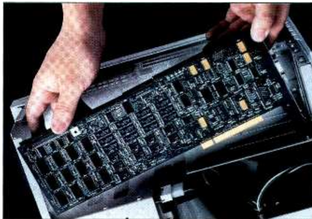
Pinnacle Genie, a 3-D digital effects system on a single PCI card.
