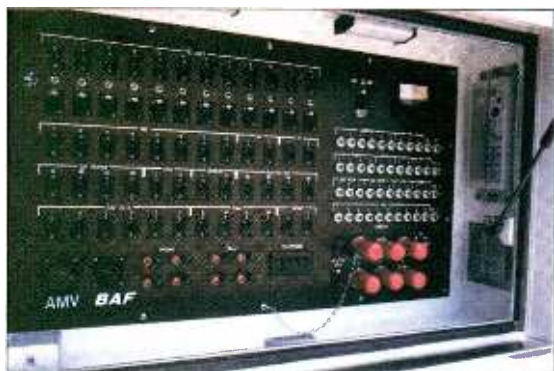
Breakout panel has lights and an intercom station with speaker on this truck owned by All Mobile Video and built by BAF. This simplifies setup and allows hands-free operation while connecting cables. A panel VU meter allows line and mic level signals to be checked easily. Switches allow pin 1 to be lifted on individual audio cables.
