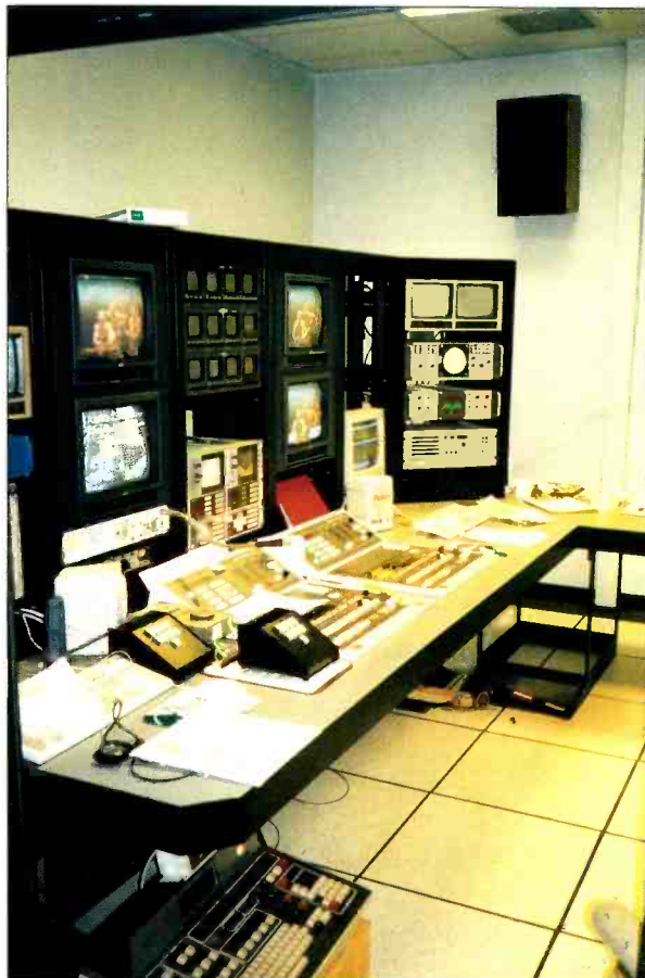
Multiple identical switchers are recommended when you need to create fully independent programming streams.
