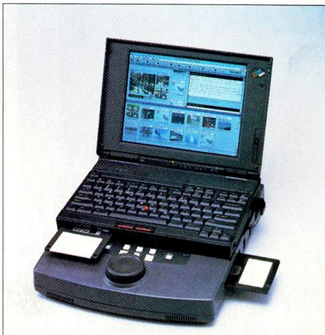
The DNE-50 provides both on-line and off-line capabilities. The unit combines a docking station with a notebook PC. A 3.5-inch magneto-optical disk drive can record 40 minutes of compressed off-line-quality video and audio material.
